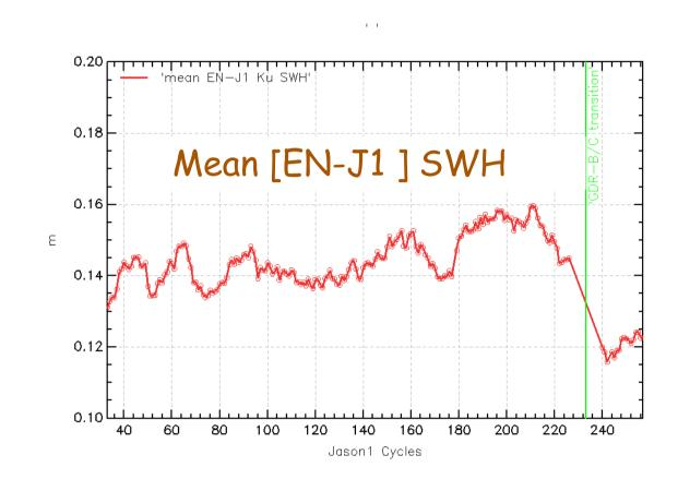
•The cycle by cycle mean of Envisat-Jason-1 SWH differences are plotted. These differences are quite stable. Envisat SWH is 15 cm higher than Jason-1 SWH. •EN/J1 Difference decreases by 3cm with Jason-1 GDRC
