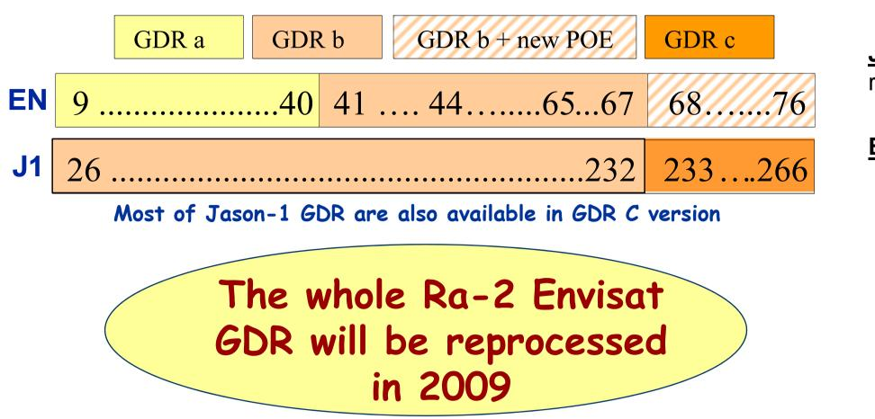
**USO anomaly:** In February 2006, the RA-2 Ultra Stable Oscillator (USO) clock frequency underwent, for an unknown reason, a strong change of behavior. The anomaly consists in a bias, superposed with an oscillating signal with an orbital period. Auxiliary files are distributed since mid 2006 allowing the users to correct the range from this anomaly. The anomaly periods are detailed beside
