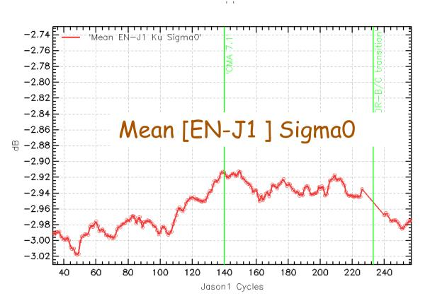
•The cycle by cycle mean of Envisat-Jason-1 differences are plotted. The mean difference between Envisat and Jason-1 Ku-band SigmaO is -2.9 dB. This mean difference has increased by 0.07dB between cycles 48 and 129 which corresponds to 0.04 dB/year. •EN/J1 difference decreases by -4.10<sup>-2</sup>dB with Jason-1 GDRC
