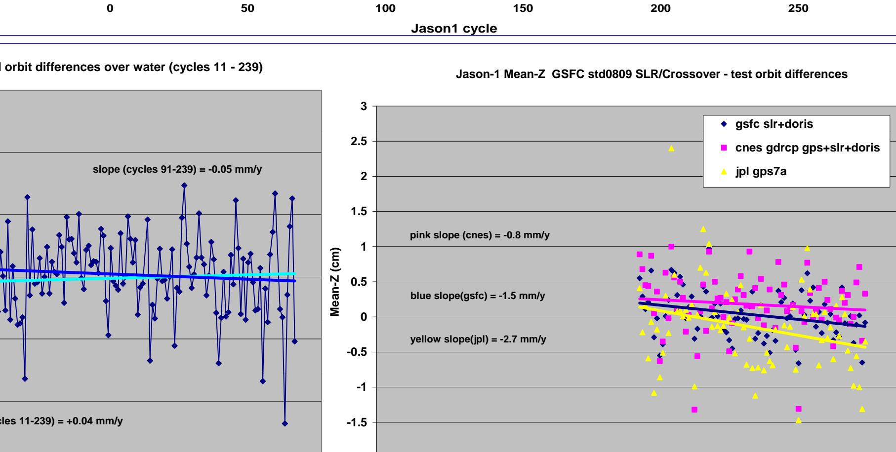
**Orbit Centering Trends in mean-Z** orbit centering contribute about 20% of that error to global MSL trend estimates. Orbit centering error appears to add about 0.4 mm/y to the MSL linear trend estimate error budget.
