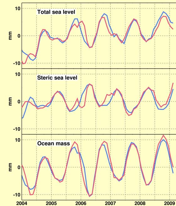
Variability in total global mean sea level and its steric and mass components. The blue lines are the observed (top) total sea level from Jason-1 and Jason-2, (middle) steric sea level from Argo, and (bottom) ocean mass from GRACE. The red lines show the inferred variability from the complementary observations computed as in (1). A 3-month boxcar smoothing is applied to each time series.
