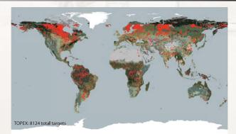
different orbit repeat pattern. However, the majority of the enhancement is due to the ERS2 altimeter being configured with a wider range window over land. Whilst this restricted the vertical precision of measurement, it greatly increases the number of targets successfully acquired. For EnviSat, even more targets are acquired, although the skewing of the instrument logic to favour ocean mode operation degrades the waveform capture over some inland water targets
