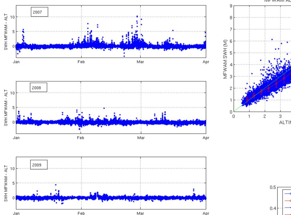
Differences between model and altimeter data 3 tropical cyclone seasons (2007, 2008, 2009). In 2007, before the intoduction of the new bogusing, differences are very high in cyclone vents.
