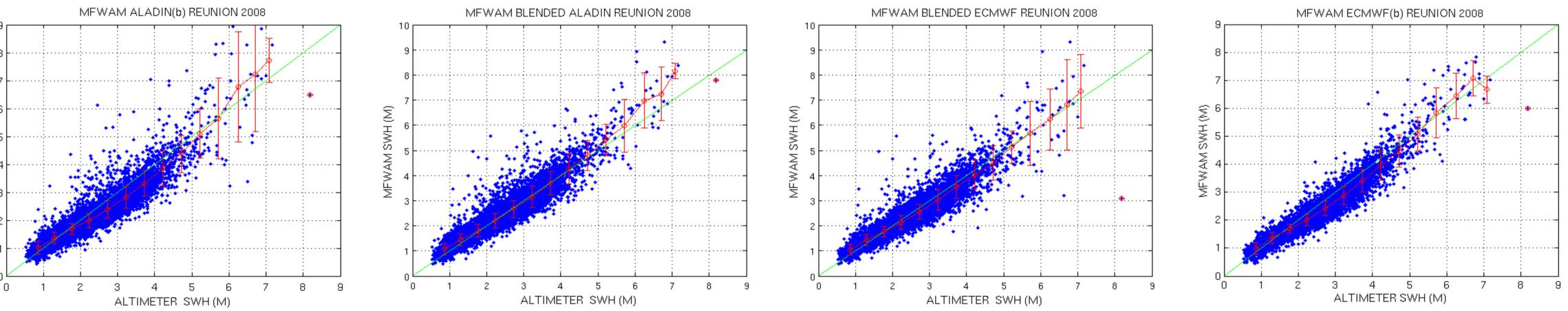
Scatter diagramm of SWH from MFWAM versus SWH from Altimeters. When using blended winds, the dispersion of the error and the error biases are significantly reduced.
