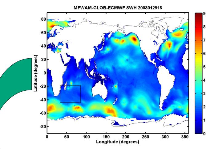
$$\frac{\partial F(f,\theta)}{\partial t} + c_g \cdot \nabla F(f,\theta) + \frac{\partial}{\partial \theta} \left[ \left( c_g \cdot \nabla \theta \right) F(f,\theta) \right] = S(f,\theta)$$
