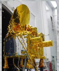
SARAL Payload Integration Module after thermal vacuum
