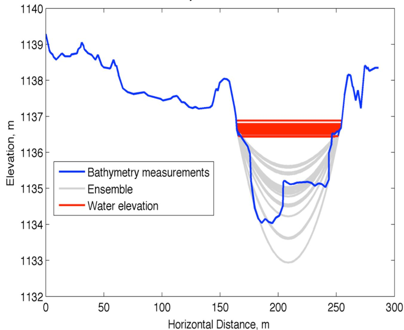
Estimated MCH Geometry, Overbanks from DTM
