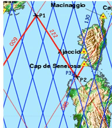
**Figure 9.1.2.** Configuration of the calibration site in Senetosa (Jason-2 groundtracks in red, EnviSat in blue).
