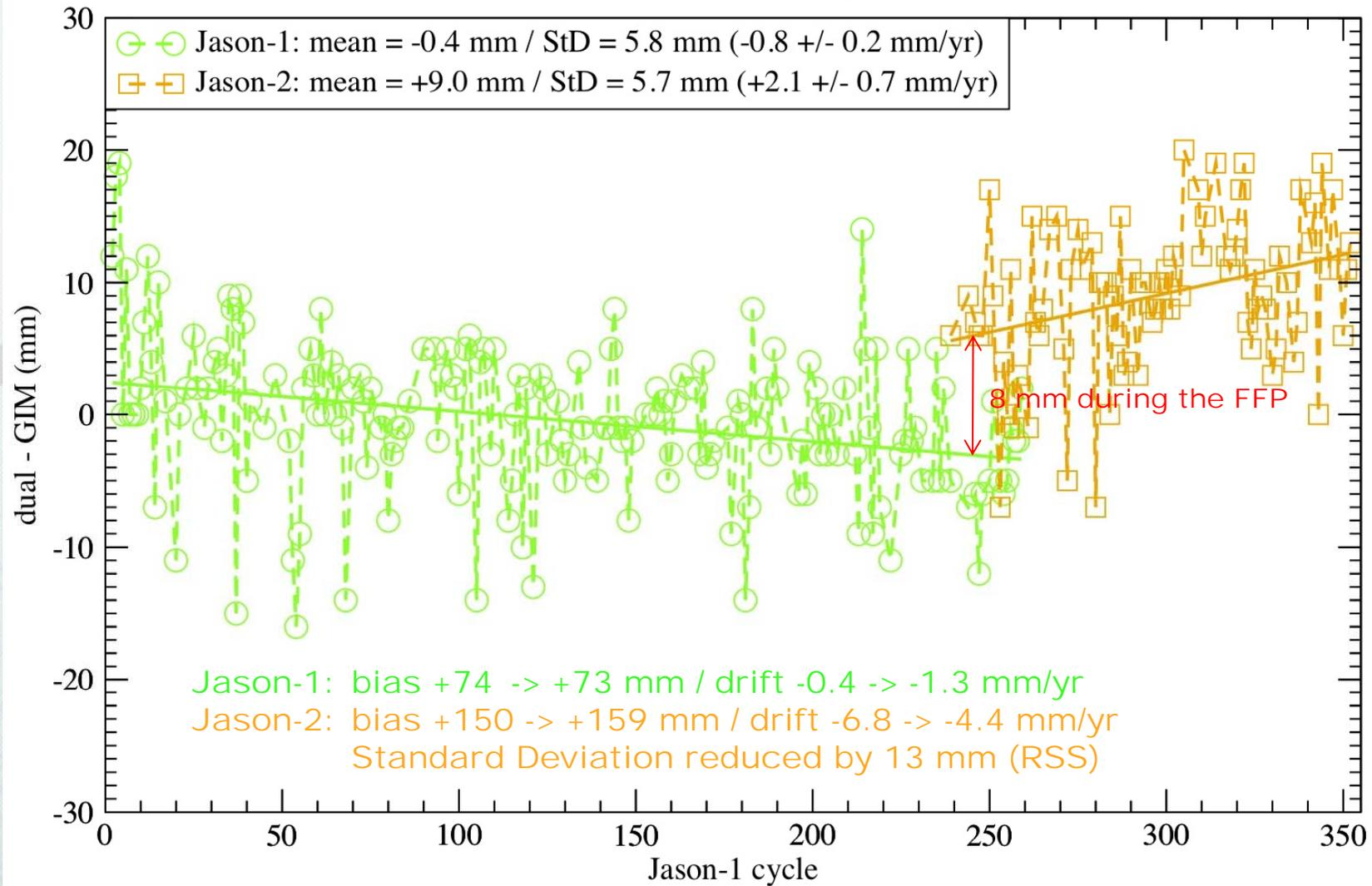
Jason-1&2 Ionospheric Path Delay (correction)
