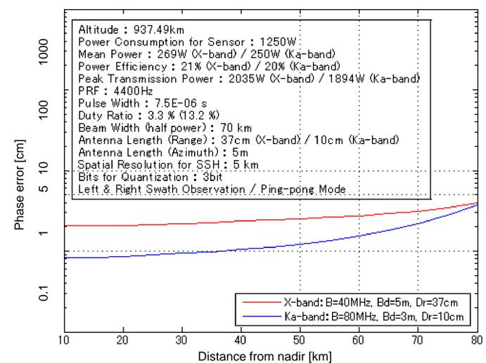
Figure 3. Calculation of phase error for X-band and Ka-band
