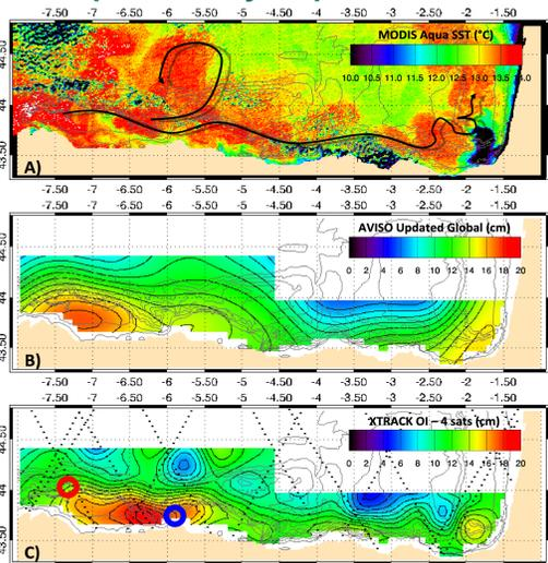
Fig. 4. Upper panel ) MODIS SST image. Middle panel) AVISO DT-MSLA Upd data. Lower panel) 55km resolution mapping - 1/16°. Bathymetry & T/P + GFO ground tracks overlaid. 1/16° grid, 55km scales.
