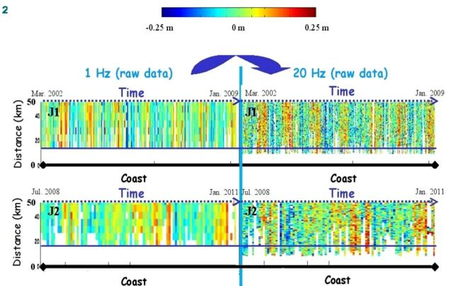
Fig. 1. Comparison of available SLA between 1Hz and 20 Hz data for Jason-1 (upper level) and Jason-2 (lower level), track 146.
