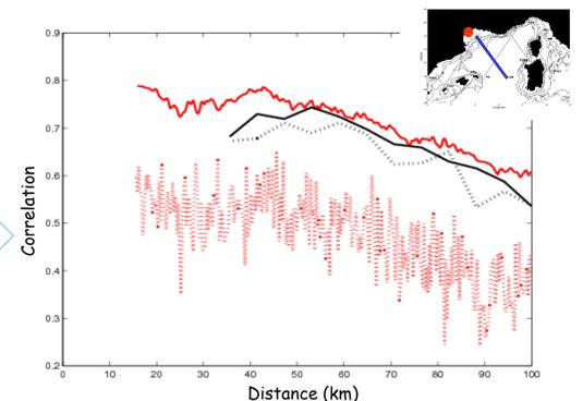
Fig. 2. Correlation between SLA raw data (solid line) and tide-gauge of Sète and between spatially filtered about 24 km (dashed line) and tide-gauge, for 1Hz SLA (in black) and 20Hz SLA (in red), for Jason-1, track 146.
