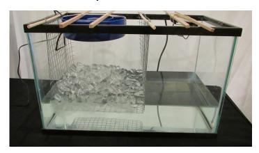
Continental Ice: To simulate melting continental ice (A), we positioned the ice in a wire mesh basket sitting slightly above the surface of the water, using a fan to improve air circulation and speed the melting of ice.
