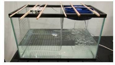
Sea Ice: To simulate melting continental ice (A), we positioned the ice in a wire mesh basket sitting on the surface of the water, using a fan to improve air circulation and speed the melting of ice.
