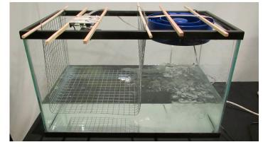
Sea Ice: To simulate melting continental ice (A), we positioned the ice in a wire mesh basket sitting on the surface of the water, using a fan to improve air circulation and speed the melting of ice.
