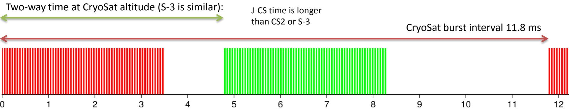
In a closed-burst SAR (CryoSat, S-3, J-CS baseline) **transmit** and **receive** are not interleaved and are not continuous. The CryoSat values of  $N = 64$  and  $PRF = 18$  kHz give a burst duration of  $\sim 3.5$  ms. But the burst-to-burst interval is  $\sim 11.8$  ms.
