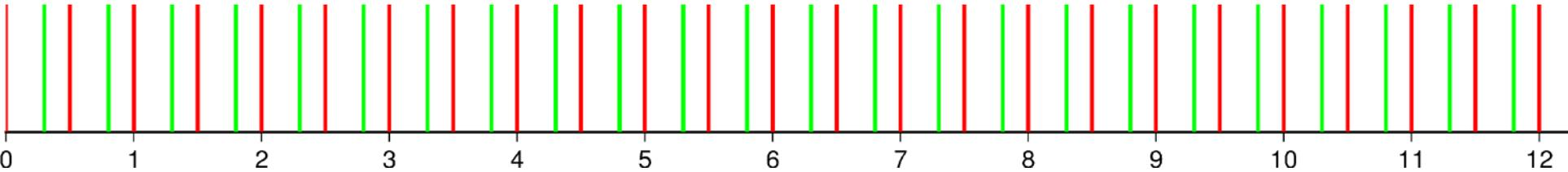
In a conventional LRM instrument, **transmit** and **receive** are *interleaved* and go on alternately, each at approximately 2 per millisecond (PRF  $\approx$  2 kHz).
