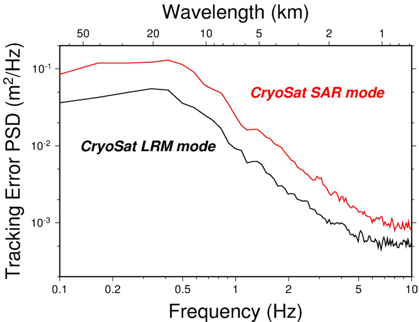
Range gate tracking errors (error in timing the digitizing of the returned radar echoes), expressed as range to the sea surface.
