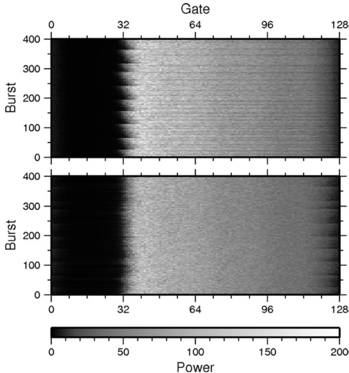
All altimeters, by design, can time the digitizing of received echoes only coarsely. If not corrected, the expected time to nadir jitters by  $\pm 2$  range gates in the waveform.
