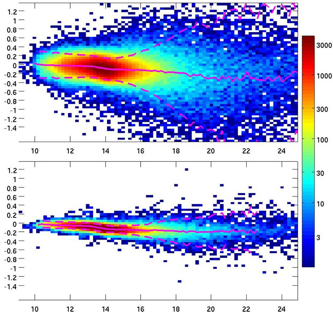
Sigma0\_Ku difference (Jason2-Jason1) as a function of Sigma0\_Ku
