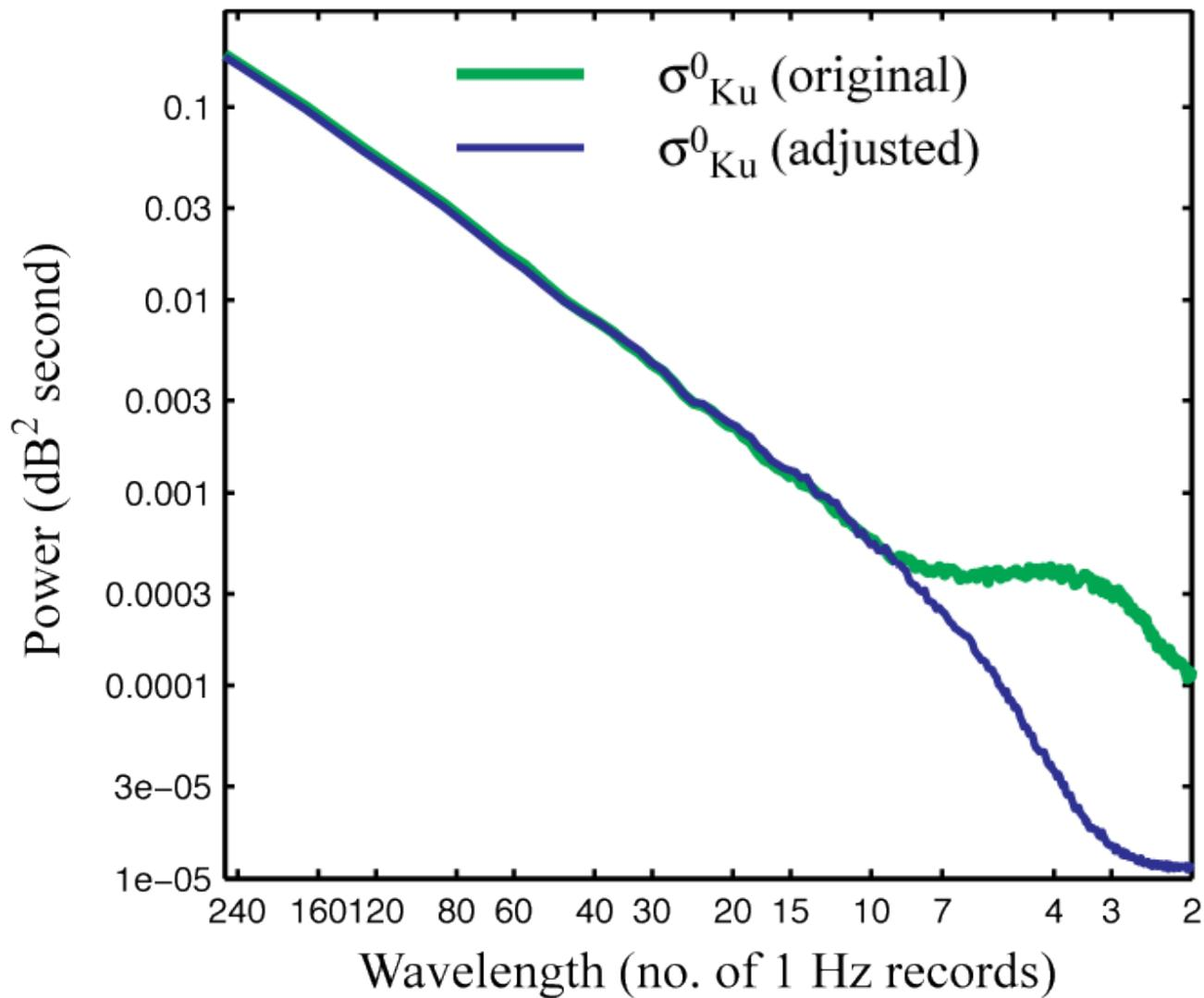
2) Mismatch between Jason-1 and Jason-2 1 Hz sigma0 values is reduced by a factor of 3 from r.m.s. difference of 0.15 dB (top) to 0.05 dB (bottom)
