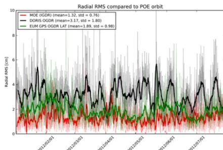
Fig. 4 Radial RMS accuracy of operational OGDR, EUM GPS OGDR LAT, and MOE orbits against Final POE orbit. Both OGDR have similar timeliness (~3 hours, cf. Fig. 6). Note that a small number of outliers in the experimental products have been removed due to issues with the onboard GPS receiver.
