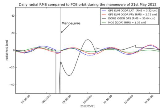
Fig. 9 Radial difference of different products compared to POD during manoeuvre
