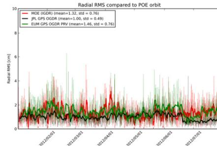
Fig. 5 Radial RMS accuracy of JPL GPS OGDR, EUM GPS OGDR PRV and IGDR orbits against Final POE(GDR) orbits. Both NRT products have similar timeliness (~5 hours, cf. Fig. 6), while IGDR product has one day lag. Note that a small number of outliers in the experimental products have been removed due to issues with the onboard GPS receiver.
