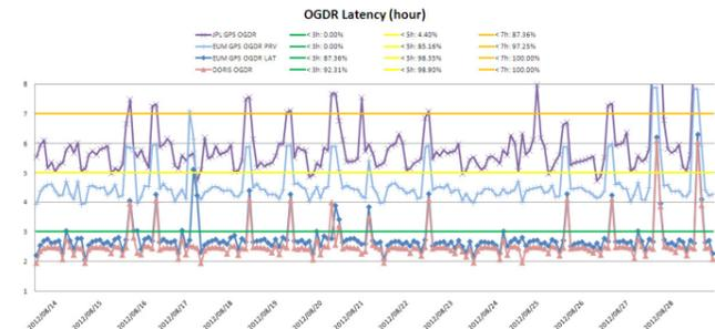
Fig. 6 Latency of all NRT OGDR products. Latency requirements are (J2GS-PROPRO-005):
