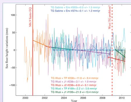
Absolute motion derived from tide gauge and altimetry data. We can see a clear difference in trend between the two gauges (on 2 different tectonic plates).
