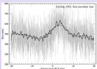
Example of along-track geoid error estimation. Along-track biases variations (altimetry derived sea surface height minus tide gauge derived sea surface height). Raw differences in grey, running-averaged (1 km) ones in black.
