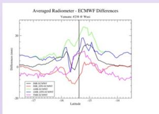
Land contamination effect on the wet tropospheric correction. The plot shows differences between radiometer (GDR or decontaminated values) and modeled values averaged along the track on successive 5 km long windows. We used Brown (2010) decontamination algorithm (EPD).
