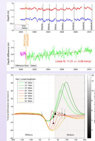
Relative motion between both tide gauges, located on both sides of the plate boundary.
