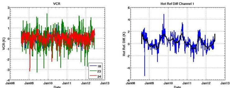
Figure 3. AMR vicarious cold reference statistic (left) and comparison to Amazon hot reference model at 18.7 GHz (right). The derived calibration is stable relative to these natural TB references.
