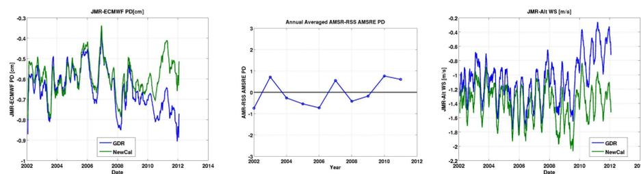
Figure 6. JMR PD compared to ECMWF (left), JMR PD compared to AMSRE PD from RSS (middle) and JMR wind speed (right) compared to the altimeter (right) after applying time variable TB correction. The PD and wind speed drifts are significantly reduced after July 2010.
