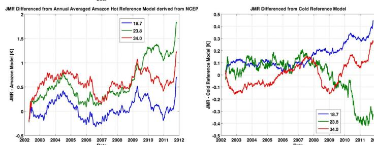
Figure 5. JMR dynamic hot reference model derived using NCEP re-analysis fields (top), JMR GDR TBs compared to hot reference model (bottom left) and JMR GDR TBs compared to cold reference model (bottom right).
