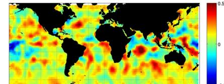
Figure 7. JMR regional PD drift from AMSR-E for 2002-2011 for GDR calibration (left) and updated calibration (right). The regional drift is reduced to << 0.5mm/yr with the updated calibration.
