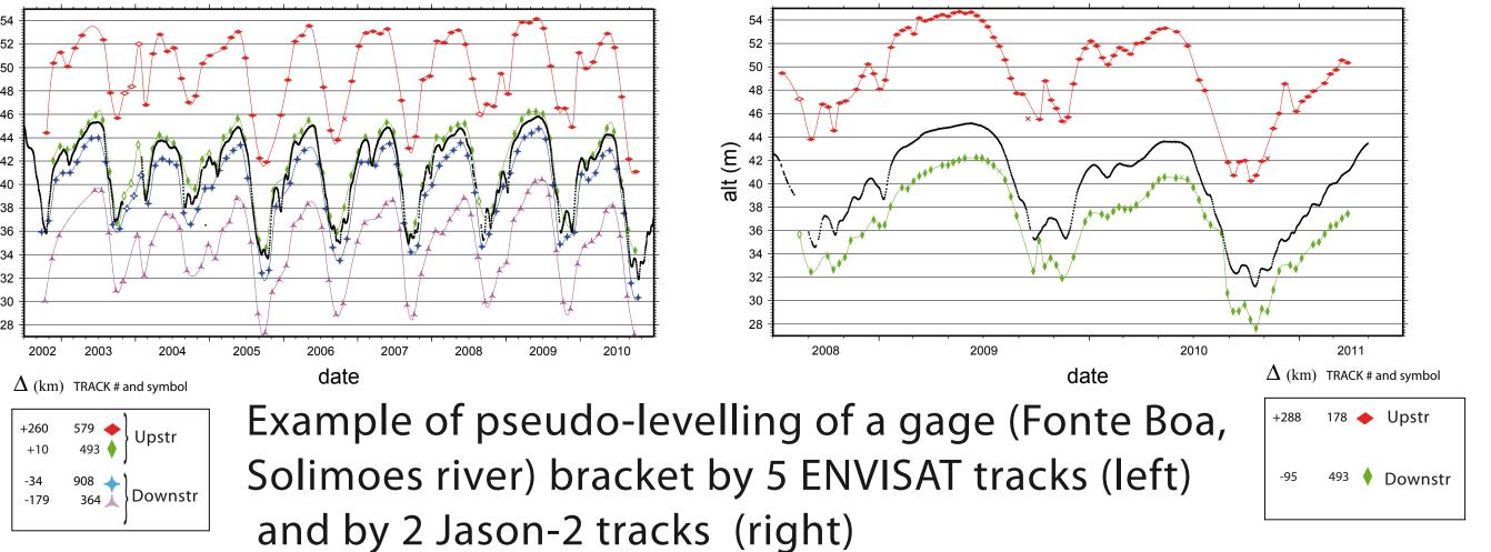
In the example shown above, the difference in absolute gage heights is due to the difference in the gage zero resulting from different altimetry bias between ENVISAT (*ice-1*) and Jason-2 (*ice-3*)
