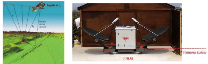
Fig.4: The procedure for transponder calibration (left) and the TUC's transponder (right).
