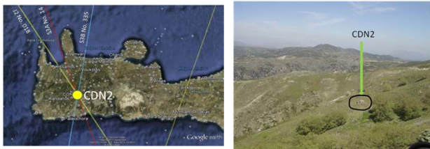
Fig.3: Altimetry missions over CDN2: S3A = red, S3B = blue, Jason-2 = yellow
