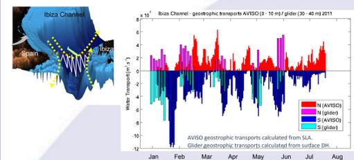
Figure 7: Surface transport across the Ibiza channel from glider and altimetry gridded fields provided by AVISO.
