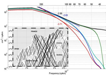
Wavenumber spectral slopes obtained from the new satellite-derived fields reveal a more realistic cascade of eddy energy.
