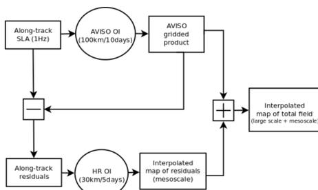
To adjust the OI parameters, sensitivity tests based on Monte-Carlo analyses were performed. The values that optimize the signal-to-noise ratio were  $L = 30$  km,  $T = 3$  days and  $\Phi = 0.7$ , with a measurement error variance of  $3 \text{ cm}^2$ .
