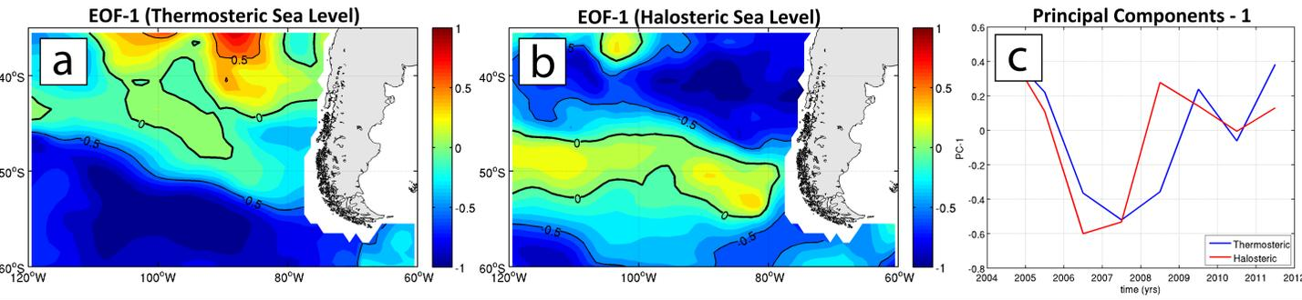
**Figure 2.** EOF-1 of the thermosteric (a) and halosteric (b) SLA and PC-1 of the thermosteric (blue curve) and halosteric (red curve) SLA explaining 50% and 55.1% of variance, respectively. The thermosteric and halosteric SLA were computed relative to 2000 db.
