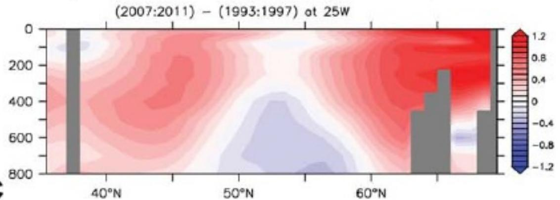
0-700m heat content change, 2007-2011 minus 1993-1997 with mean surface circulation shows heat added in boundary currents of subpolar gyre
