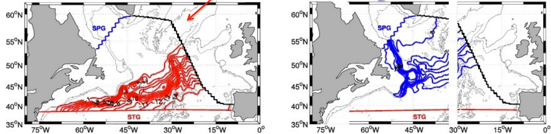
As the subpolar gyre weakens, the flow south of 50N decreases less than the flow north of 50N decreases... **there is less competition for the warmer southern branch of NAC less dilution of the warm, saline waters** (in this model, the northward AMOC transport has not increased but its heat and salt transport have)
