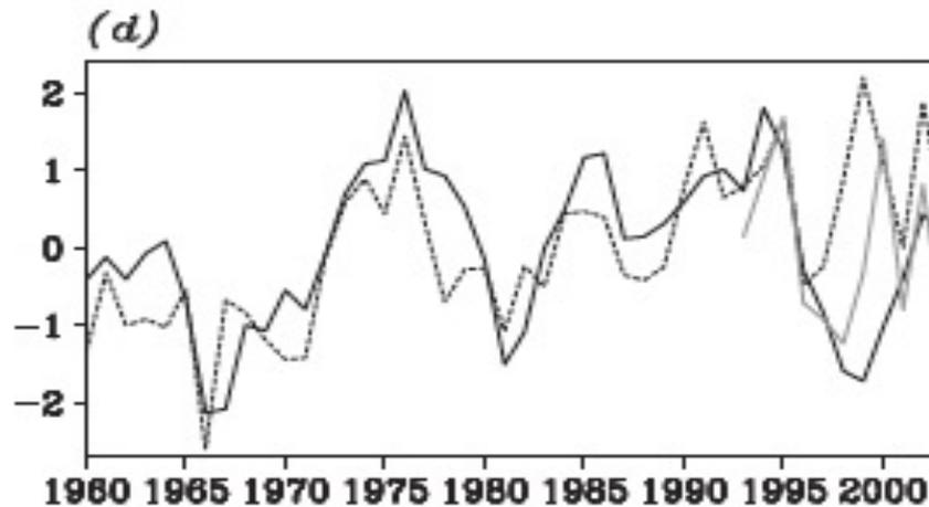
SSH anomalies develop  $\sim 2$  years before reaching Gulf Stream and changing its latitude, propagating as a Rossby wave guided by the boundary current extension. OFES model *Sasaki & Schneider OM 2010*
