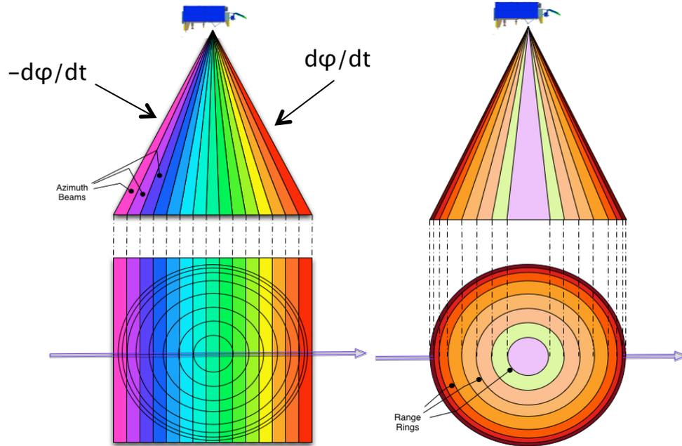
Azimuth Processing provides Complex Stack Data (L1B-S) and Multi-looked echoes (L1B)
