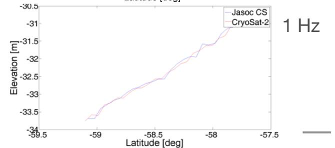
**Verification:** Example of Jason-CS P4 GPP Verification prior interleaved using CryoSat data adapted to Jason-CS
