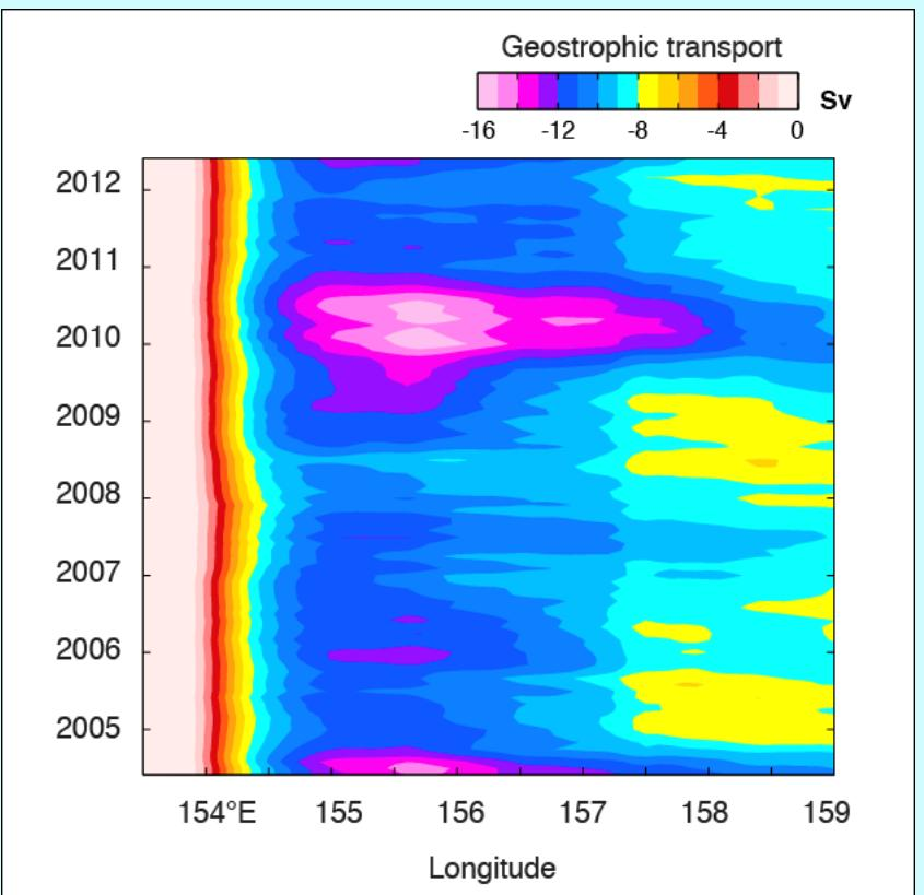
0-800 m geostrophic transport west of 155.5°E computed with XBT/altimetry data shows  $\pm 1.3$  Sv variability at interannual time scales. ENSO signature seen in EAC transport anomalies is more evident during strongest El Niño and La Niña events.
