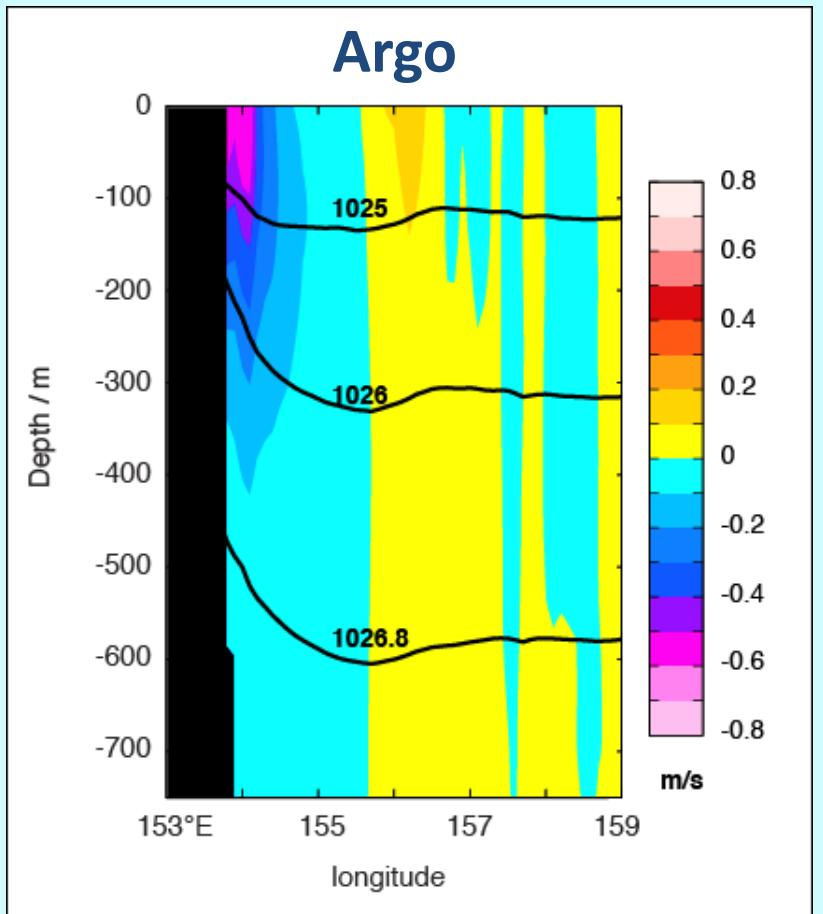
The core of the EAC is of greater magnitude using XBT than Argo.
