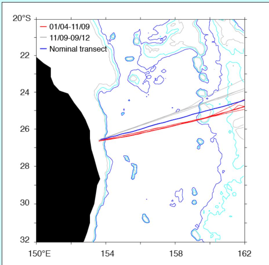
XBT temperature profiles along each track are projected onto a nominal transect using Argo map of temperature.
