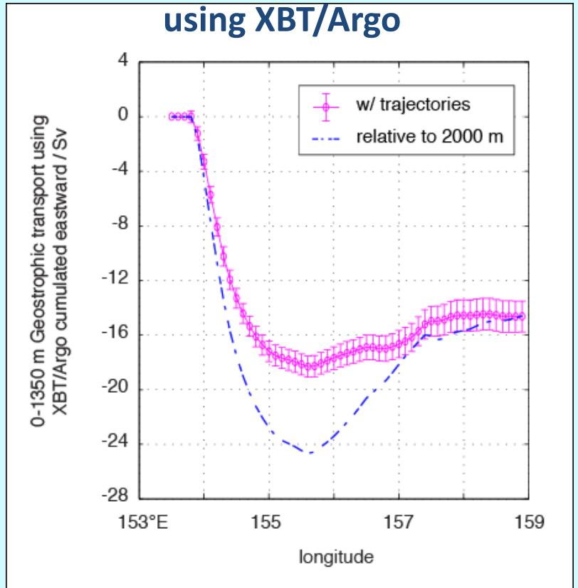
Argo trajectories show less negative velocity than XBT/Argo velocity at 1000/2000 m. Trajectories “feel” the equatorward undercurrent observed in Mata et al. (2000). 0-1350 m EAC transport west of 155.6°E using XBT/Argo w/ ref velocity from trajectories is 18.3 Sv, 6.3 Sv lower than using a level of no motion at 2000 m.
