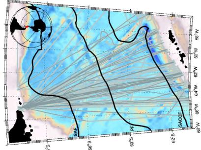
**Drake Passage transects** (gray lines) with climatological positions of the Subantarctic Front, Polar Front, and Southern ACC and Southern ACC Front (Orsi et al., 1995). Tan hues represent depths < 2600 m and transition to blue hues in the deeper parts of the passage.
