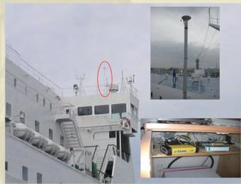
*New Camellia* (19,961 Gross Tons) with RTK GPS (NetR5, Trimble), and her mean route in the Tsushima Strait (bathymetry C.I. 20m).
