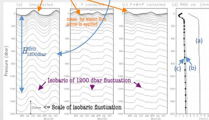
Fig. 4 Isobaric surface fluctuation for global ocean (66° S - 66° N). The way to detect the isobaric surface of 1200 dbar is shown for example.
