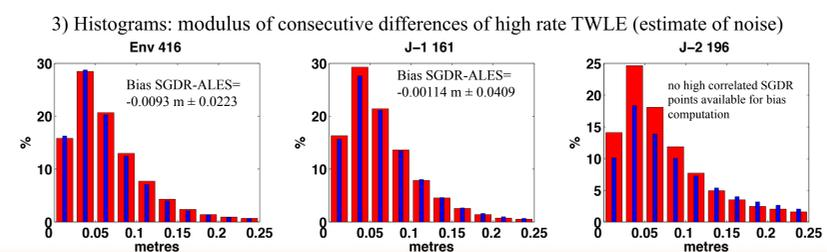
TWLE retrievals are validated against tide gauge values from Trieste, using all the available cycles for each satellite track. Raw high-rate data from ALES and standard product (SGDR) are compared with CTOH post-processed 1-Hz coastal altimetry product.
