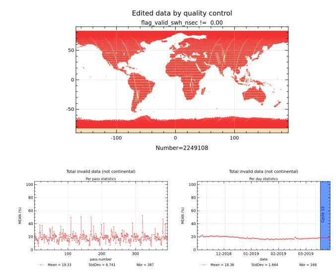
The figure on the left represents rejected values based on the editing criteria listed in Table 4.1. The map shows the SWH values of rejected points in colour. When this representation is not possible (masked points, non-computed values) points are represented in black.
