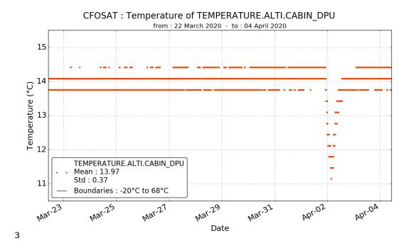
CFOSAT : Temperature of TEMPERATURE.ALTI.CABIN\_DPU Moy = 13.9667 -- Ect = 0.3700 -- Number = 138526
