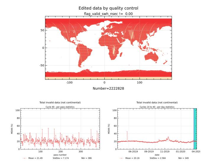
The figure on the left represents rejected values based on the editing criteria listed in Table 9.1. The map shows the SWH values of rejected points in colour. When this representation is not possible (masked points, non-computed values) points are represented in black.
