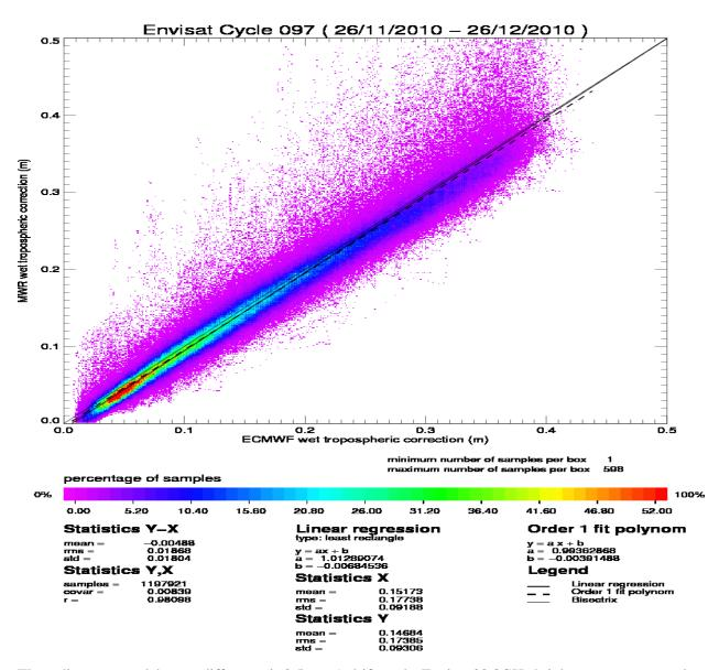
The radiometer-model mean difference is 0.5 cm. A drift on the Envisat 23.8GHz brightness temperature has been detected and has to be monitored on the long term. Note that the neural algorithm is now implemented on Envisat.
