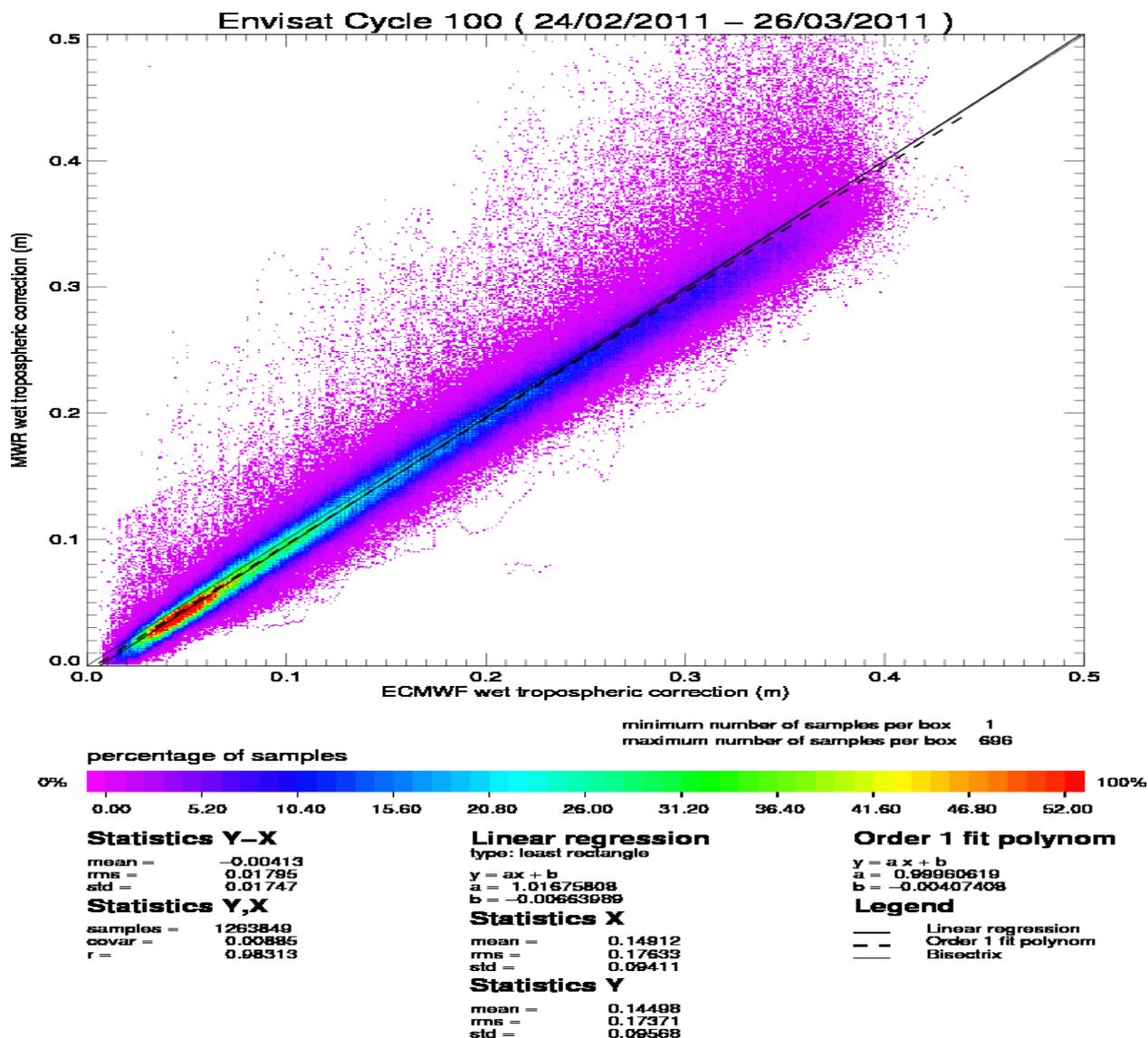
The radiometer-model mean difference is 0.4 cm. A drift on the Envisat 23.8GHz brightness temperature has been detected and has to be monitored on the long term. Note that the neural algorithm is now implemented on Envisat.
