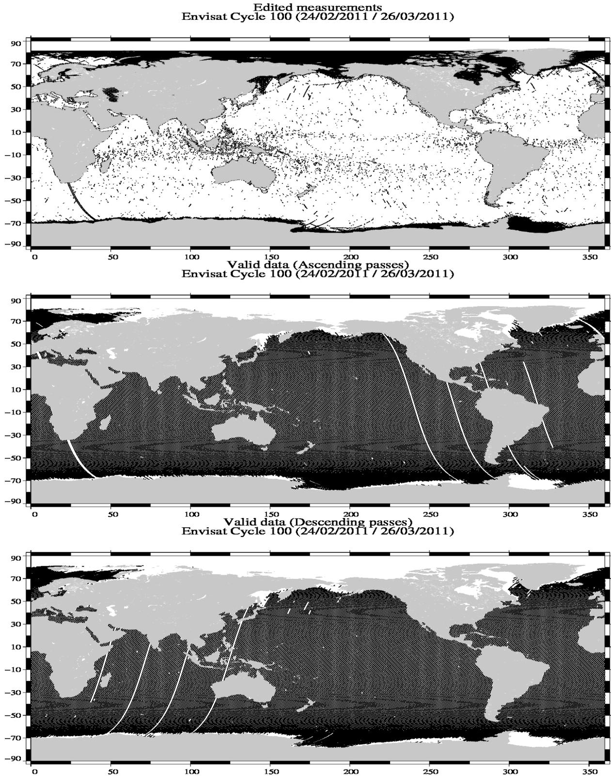
Wet areas appear in the plot of removed data. Similar features are observed with other altimeters (T/P, Jason) mainly due to rain contamination.
