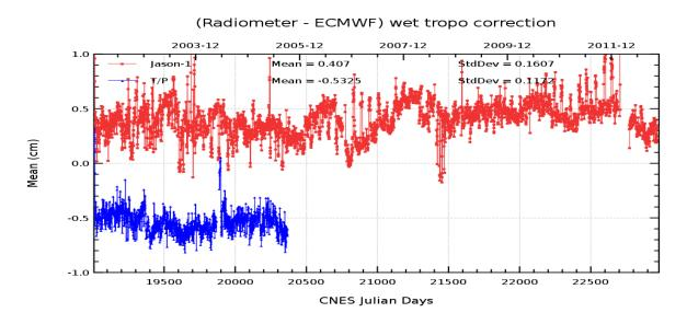
The figure below shows the mean of wet troposphere correction (radiometer - ECMWF) difference by pass.
