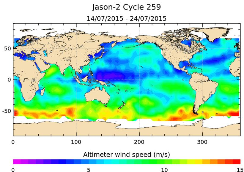
FIGURE 9 – Altimeter wind speed for cycle 259.
