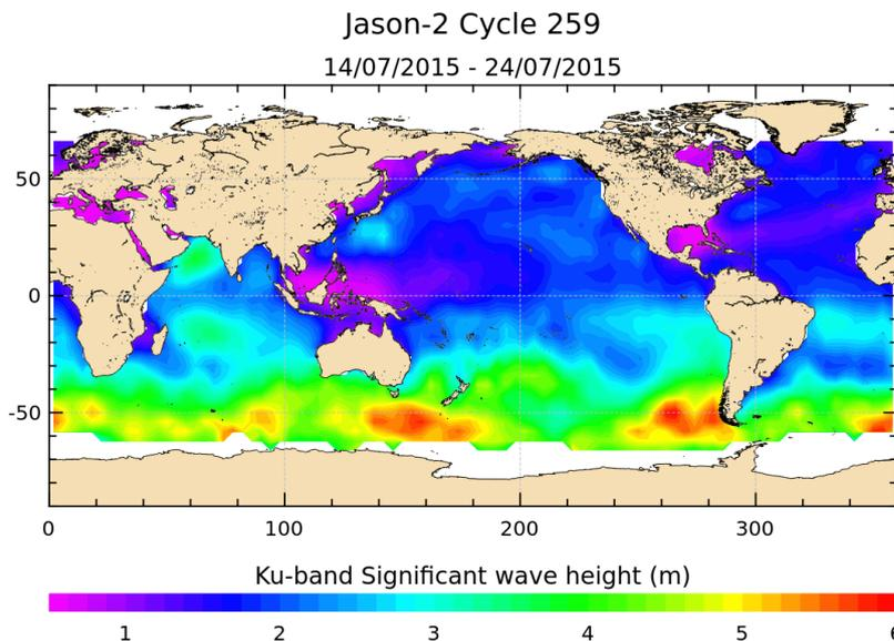
FIGURE 5 – Significant wave height for cycle 259.
