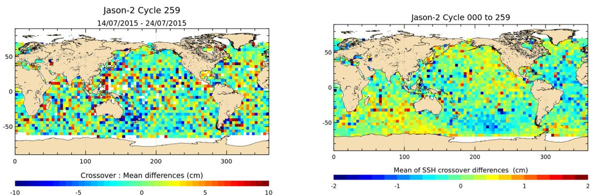
FIGURE 12 – Mean SSH at crossovers for cycle 259 (left) and over the whole Jason-2 period (right).
