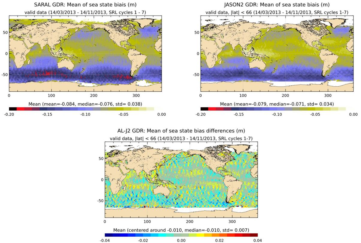
Figure 46: Average map of sea state bias for Saral/AltiKa (left) and Jason-2 (right) cycles 1 to 7. Difference map of gridded Saral and Jason-2 sea state bias for cycles 1 to 7.
