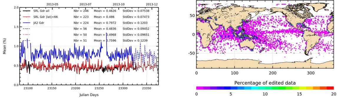
Figure 18: Percentage of edited measurements by sea surface height criterion. Left: Daily statistics for Saral/Altika (all latitudes: black, limited to 66° latitude: red) and Jason-2 (blue). Right: Map over a 8 months period (cycles 1 to 7).
