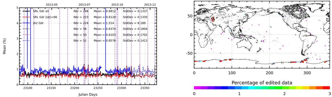
Figure 19: Percentage of edited measurements by sea level anomaly criterion. Left: Daily statistics for Saral/Altika (all latitudes: black, limited to 66° latitude: red) and Jason-2 (blue). Right: Map over a 8 months period (cycles 1 to 7).
