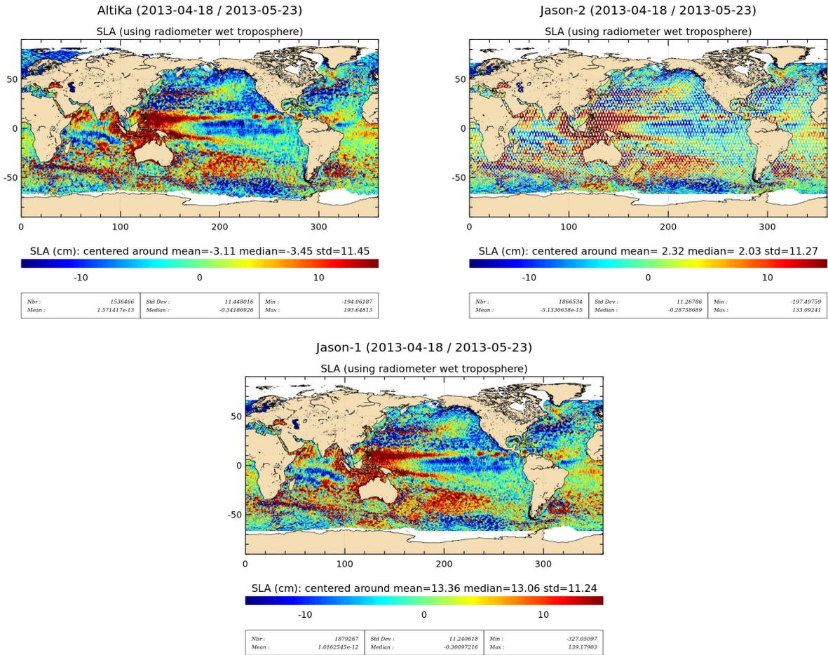
Figure 60: Map of (centered) SLA for Saral/AltiKa (top left), Jason-2 (top right) and Jason-1 (bottom) GDR data for Saral/AltiKa cycle 2.
