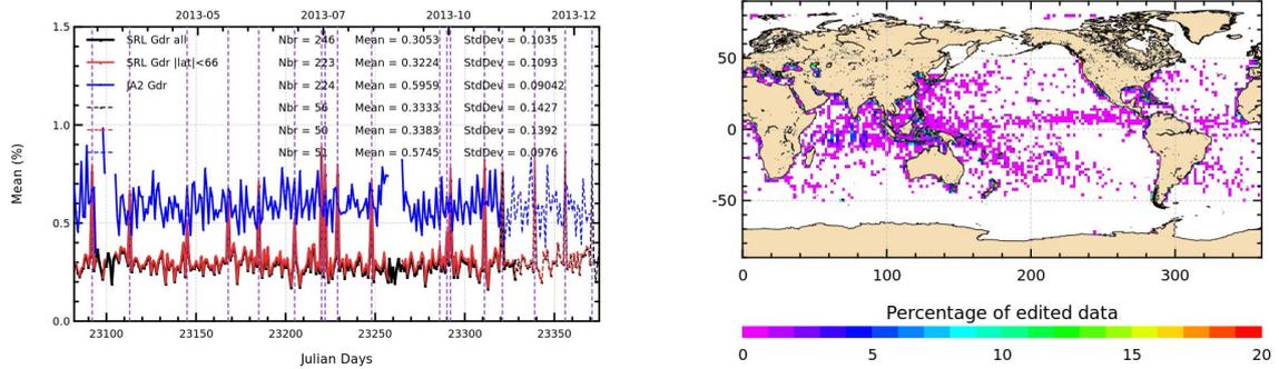
Figure 15: *Percentage of edited measurements by square off-nadir angle criterion. Left: Daily statistics for Saral/AltiKa (all latitudes: black, limited to 66° latitude: red) and Jason-2 (blue). Lilac vertical lines indicate days with maneuvers on Saral/AltiKa. Right: Map over a 8 months period (cycles 1 to 7).*
