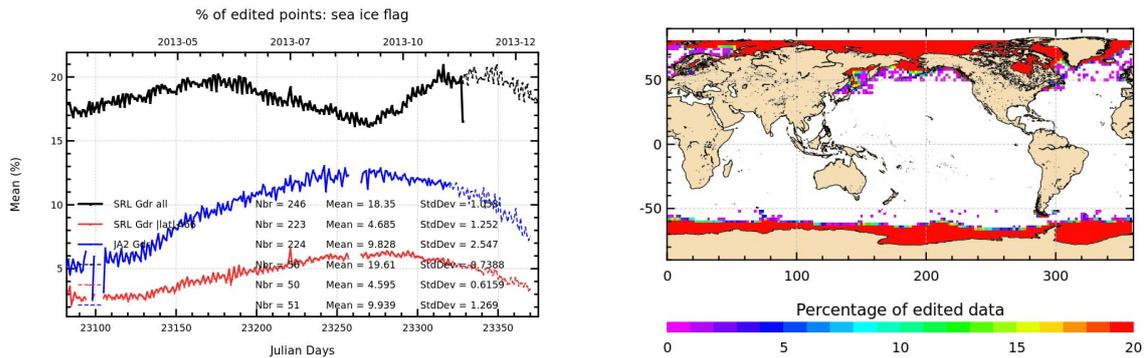
Figure 6: Percentage of edited measurements by ice flag criterion. Left: Daily statistics (plain lines: GDR, dotted lines: IGDR) for Saral/AltiKa (all latitudes: black, limited to  $66^\circ$  latitude: red) and Jason-2 (blue). Right: Map over a 8 months period (cycles 1 to 7).
