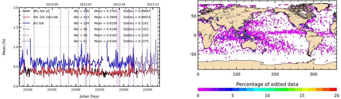
Figure 12: Percentage of edited measurements by Sigma0 criterion. Left: Daily statistics for Saral/AltiKa (all latitudes: black, limited to 66° latitude: red) and Jason-2 (blue). Lilac vertical lines indicate days with maneuvers on Saral/AltiKa. Right: Map over a 8 months period (cycles 1 to 7).
