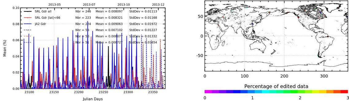
Figure 17: *Percentage of edited measurements by ocean tide criterion. Left: Daily statistics for Saral/AltiKa (all latitudes: black, limited to 66° latitude: red) and Jason-2 (blue). Right: Map over a 8 months period (cycles 1 to 7).*
