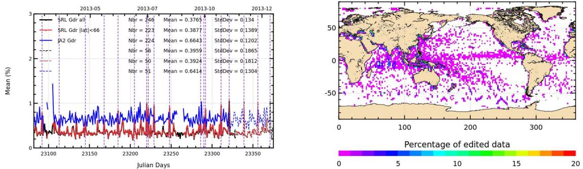
Figure 11: Percentage of edited measurements by SWH criterion. Left: Daily statistics (plain lines: GDR, dotted lines: IGDR) for Saral/AltiKa and Jason-2 (blue). Lilac vertical lines indicate days with maneuvers on Saral/AltiKa. Right: Map over a 8 months period (cycles 1 to 7).
