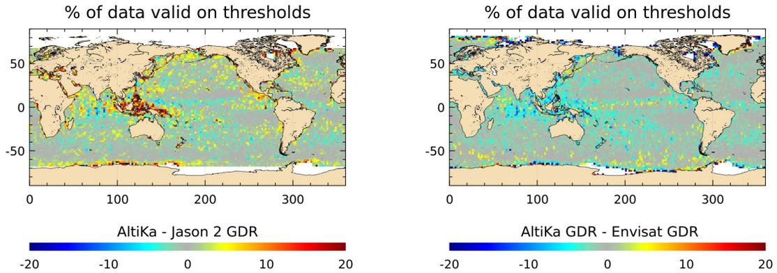
Figure 23: Percentage of difference of valid data for Saral (left) and Jason-2 (right). Saral cycles 1 to 3, Jason-2 over the same period. Envisat for the same period, but 3 years earlier.
