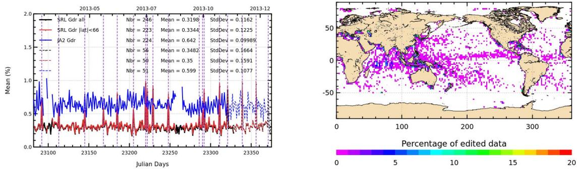
Figure 16: Percentage of edited measurements by sea state bias criterion. Left: Daily statistics for Saral/AltiKa (all latitudes: black, limited to 66° latitude: red) and Jason-2 (blue). Lilac vertical lines indicate days with maneuvers on Saral/AltiKa. Right: Map over a 8 months period (cycles 1 to 7).
