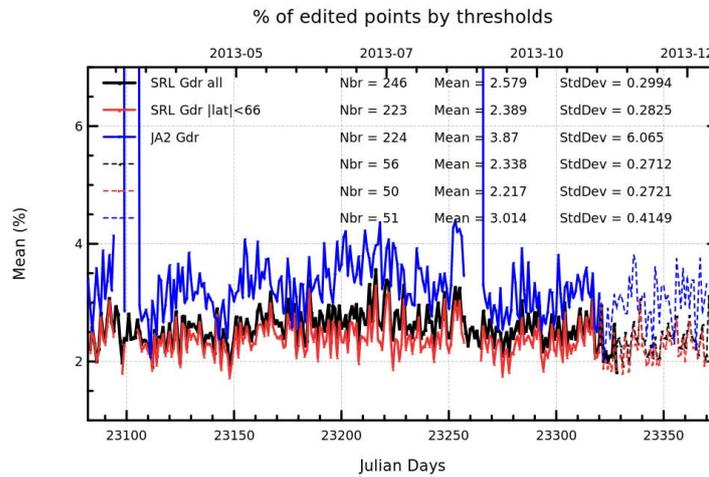
Figure 8: Daily statistics of percentage of edited measurements by threshold criteria (plain lines: GDR, dotted lines: IGDR) for Saral/AltiKa (all latitudes: black, limited to  $66^\circ$  latitude: red) and Jason-2 (blue).
