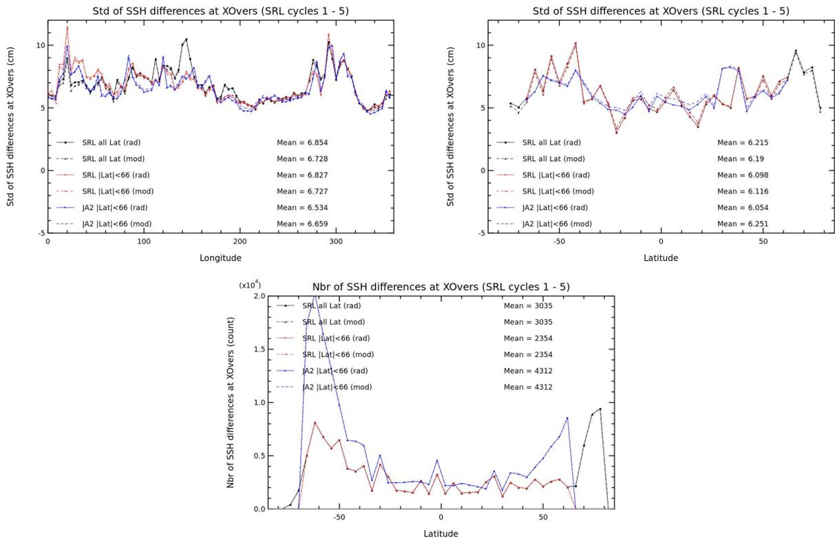
Figure 56: Std of SSH crossover differences for Saral/AltiKa and Jason-2 GDR per 4° longitude (left) and latitude (right) bands for Saral cycles 1 to 5. Bottom: Number of SSH crossover differences for Saral/AltiKa and Jason-2 GDR per 4° latitude bands.
