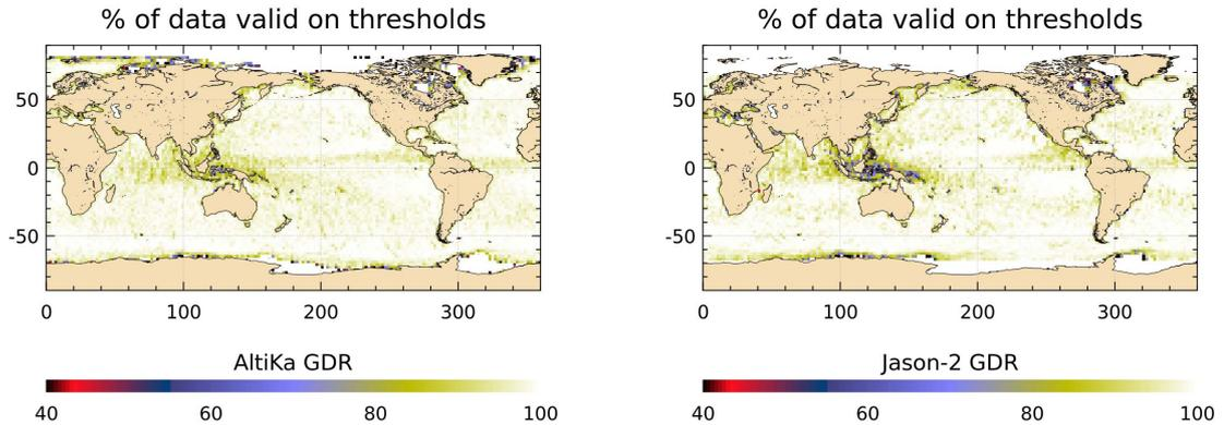
Figure 21: Percentage of valid data for Saral (left) and Jason-2 (right). Saral cycles 1 to 3, Jason-2 over the same period.
