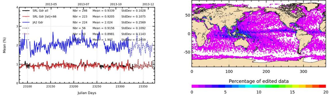
Figure 13: Percentage of edited measurements by 40 Hz Sigma0 standard deviation criterion. Left: Daily statistics for Saral/AltiKa (all latitudes: black, limited to 66° latitude: red) and Jason-2 (blue). Right: Map over a 8 months period (cycles 1 to 7).
