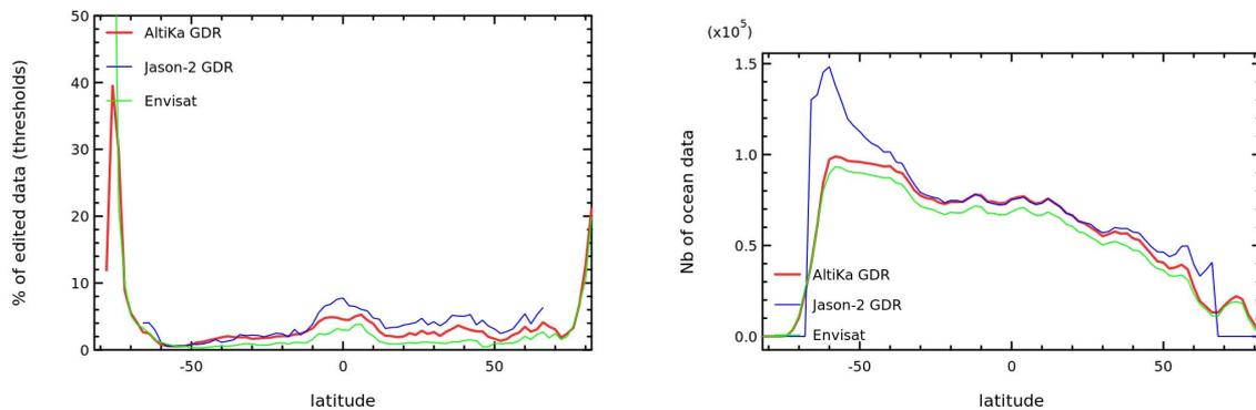
Figure 22: Percentage of edited data in function of latitude bands (left). Number of ocean data in function of latitude bands (right). Latitude bands have a width of  $2^\circ$ . Saral cycles 1 to 3, Jason-2 over the same period. Envisat for the same period, but 3 years earlier.
