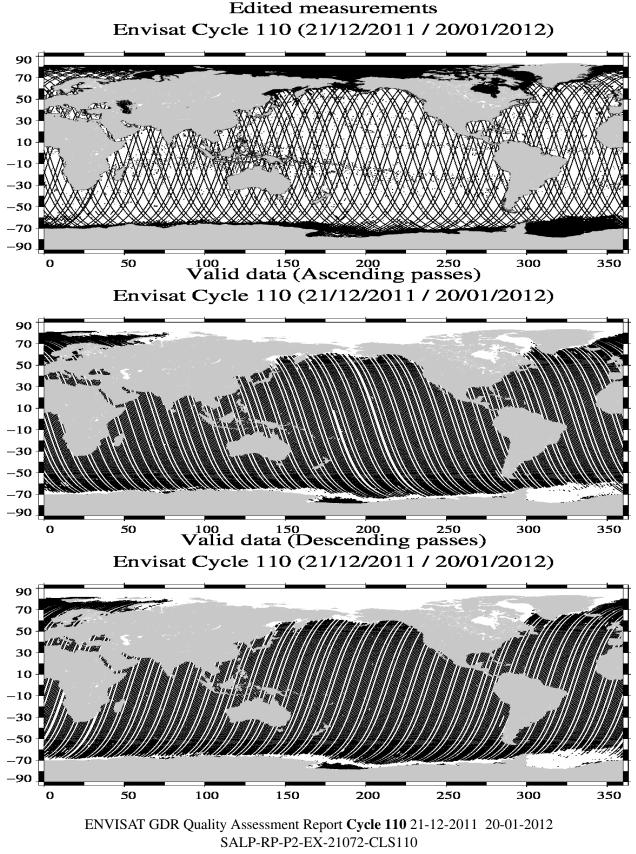
Wet areas appear in the plot of removed data. Similar features are observed with other altimeters (T/P, Jason) mainly due to rain comtamination.
