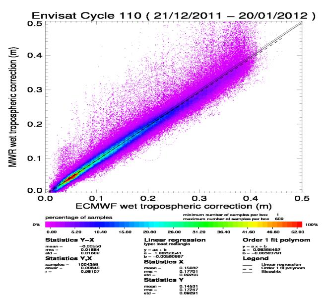
The radiometer-model mean difference is 0.6 cm. A drift on the Envisat 23.8GHz brightness temperature has been detected and has to be monitored on the long term. Note that the neural algorithm is now implemented on Envisat.
