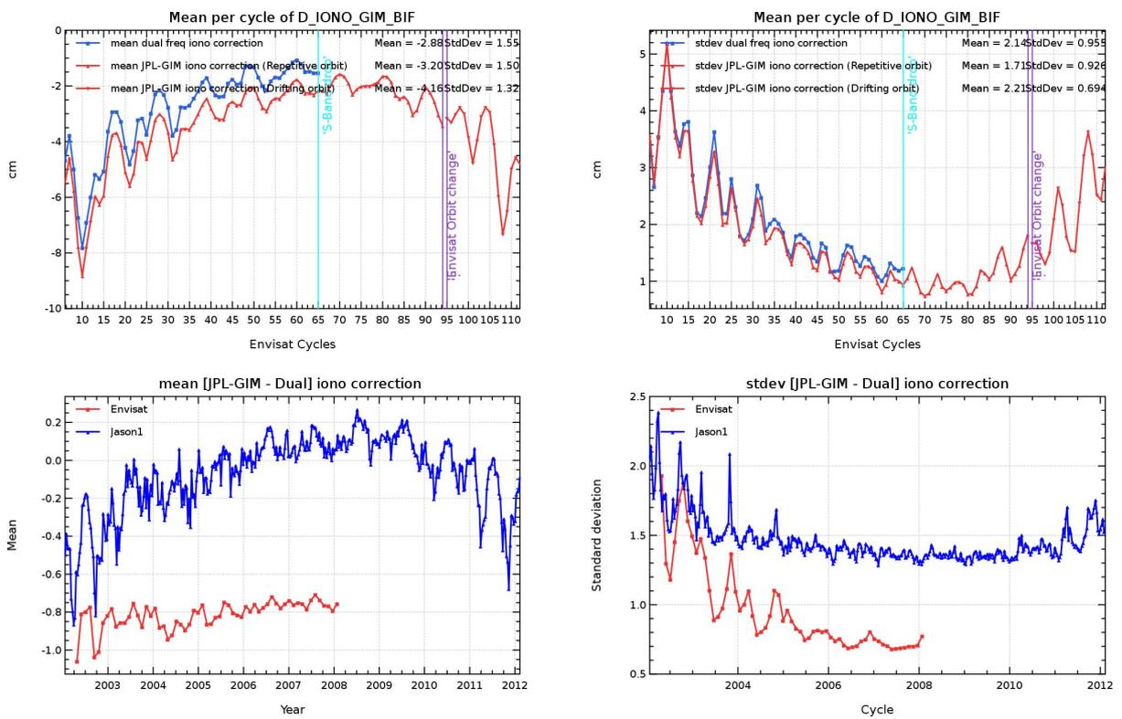
Figure 19: Comparison of global statistics of Envisat dual-frequency and JPL-GIM ionosphere corrections (cm). **Top**) Mean and standard deviation per cycle of Dual Frequency and GIM correction. **Bottom**) Mean and standard deviation of the differences for Envisat and Jason-1
