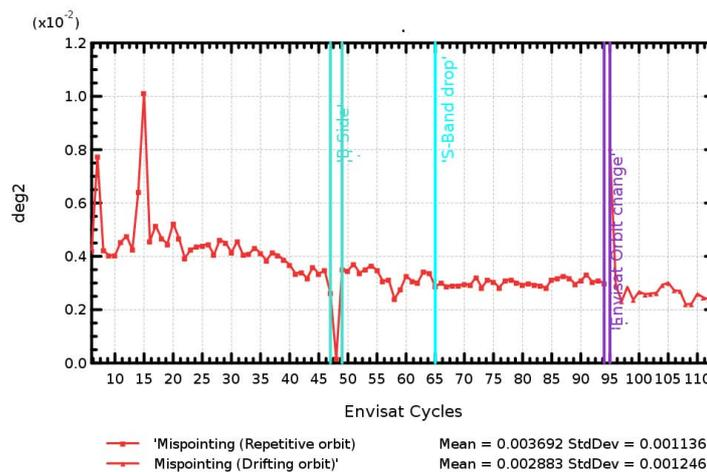
Figure 12: Mean per cycle of the square of the off-nadir angle deduced from waveforms (deg<sup>2</sup>).
