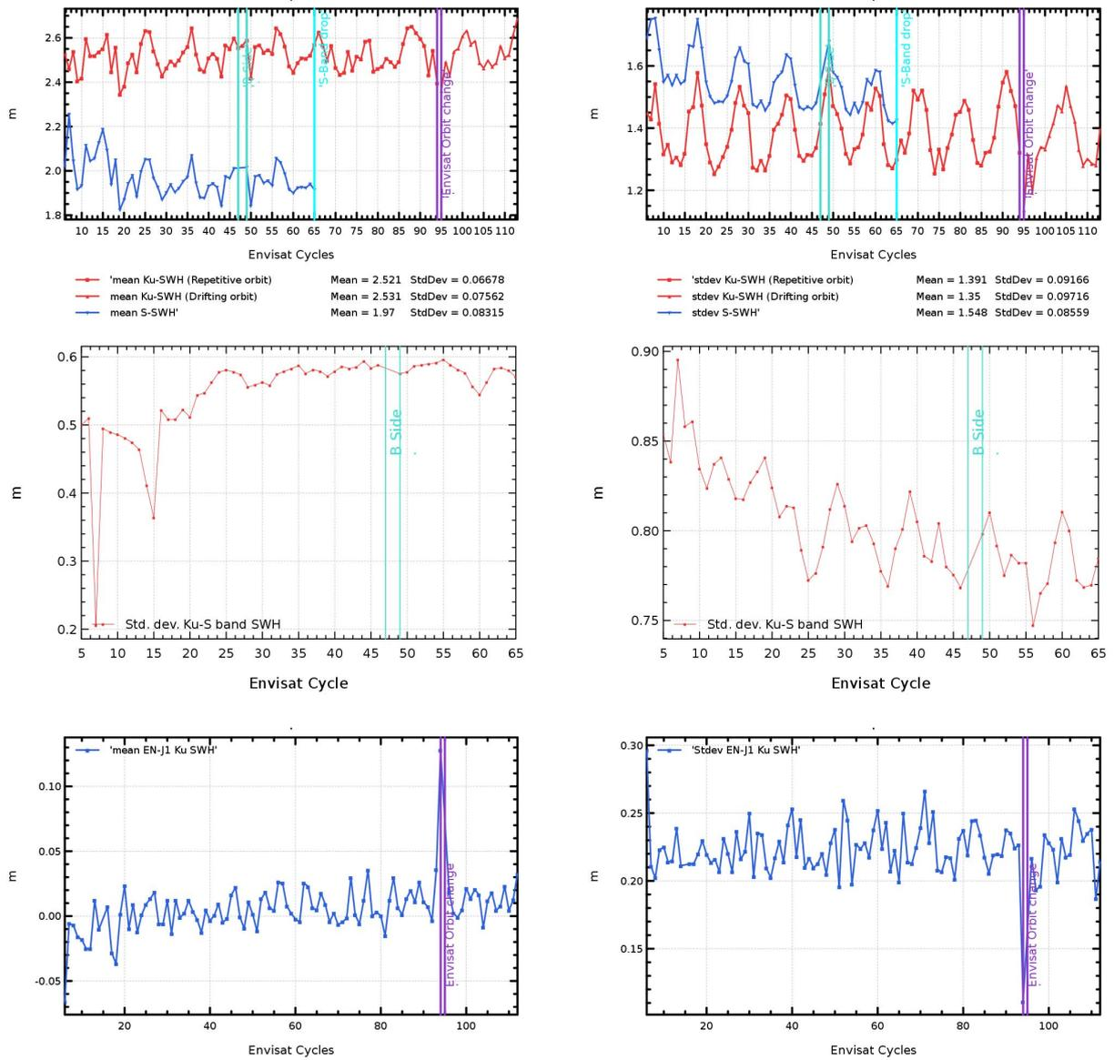
Figure 14: Global statistics (m) of Envisat Ku and S SWH **top)** Mean and Standard deviation. **Middle:** Mean and standard deviation of Ku-S band SWH **bottom)** Mean Envisat-Jason-1 Ku SWH differences at 3h EN/J1 crossovers.
