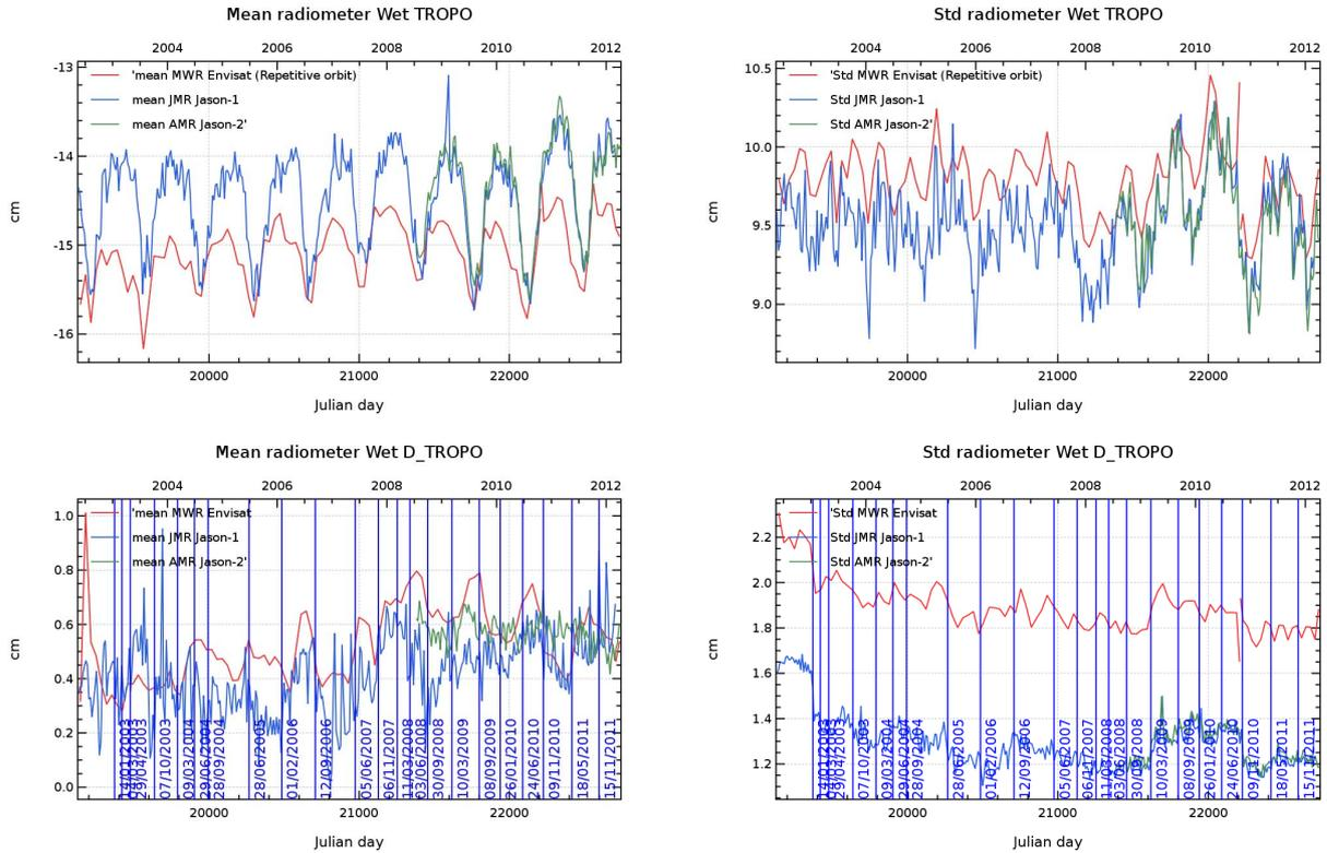
Figure 21: Comparison of global statistics of Envisat MWR and ECMWF wet troposphere corrections (cm). **top)** Mean and standard deviation per cycle of MWR, JMR and AMR corrections **Bottom)** Mean and standard deviation per cycle of the differences versus ECMWF model. Vertical lines represent the major events.
