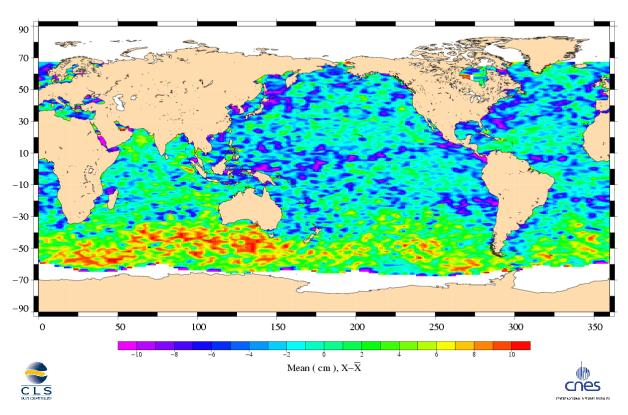
SWH KU differences Topex (Cycle 362) – Jason (Cycle 019) The scatter plot between Jason-1 and TOPEX Ku SWH measurements is given on the following figure:
