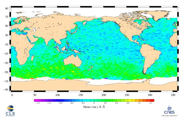
Altimeter ionospheric correction differences Topex (Cycle 362) – Jason (Cycle 019) The scatter plot between Jason-1 and TOPEX dual-frequency ionosphere corrections is given on the following figure:
