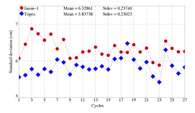
Sea Level Anomaly (SLA) statistics are computed from repeat-track analysis. The plot below gives the SLA standard deviation for each cycle over the whole data set (shallow waters are excluded).
