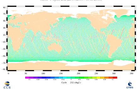
Square of the off nadir angle from waveforms Jason–1 Cycle 232 (23/04/2008 / 03/05/2008)
