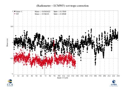
The figure below shows the mean of wet troposphere correction (radiometer - ECMWF) difference by pass.
