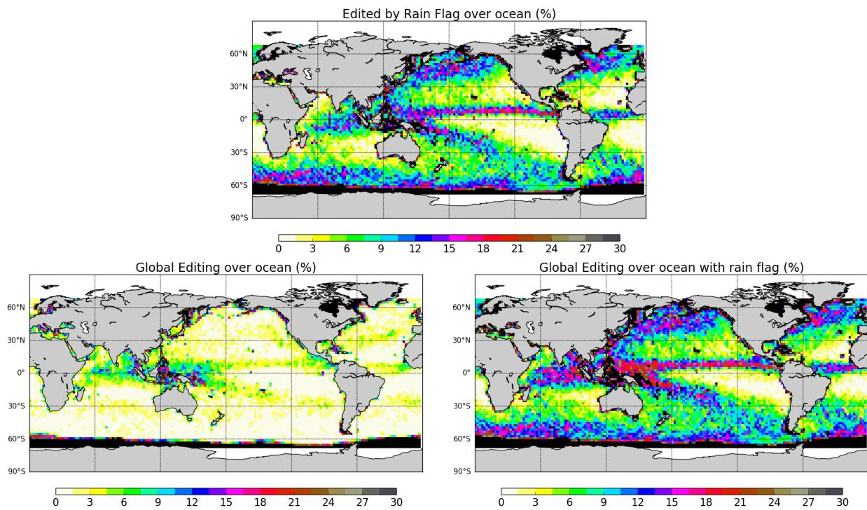
*Figure 7 – Top: Percentage of edited measurements by altimeter rain flag criterion. Bottom left: Map of global edited measurements without considering the rain flag. Bottom right: Map of global edited measurements using all criteria and considering the rain flag. All figures are computed over ocean and from cycle 62 to 98.*
