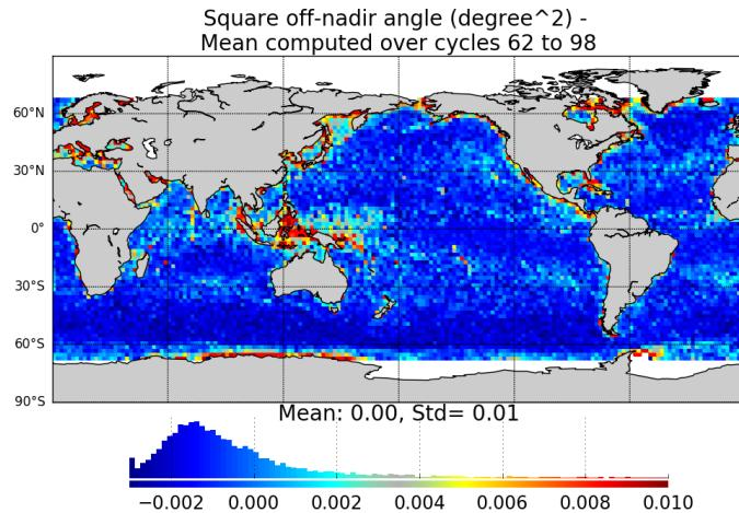
*Figure 25 – Map of the square off-nadir angle for Jason-3 averaged over cycles 62 to 98.*
