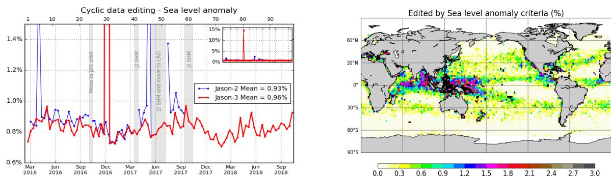
*Figure 19 – Percentage of edited measurements by sea level anomaly threshold criterion. Left: Cycle per cycle monitoring compared with Jason-2. Right: Jason-3 averaged map from cycle 62 to 98.*
