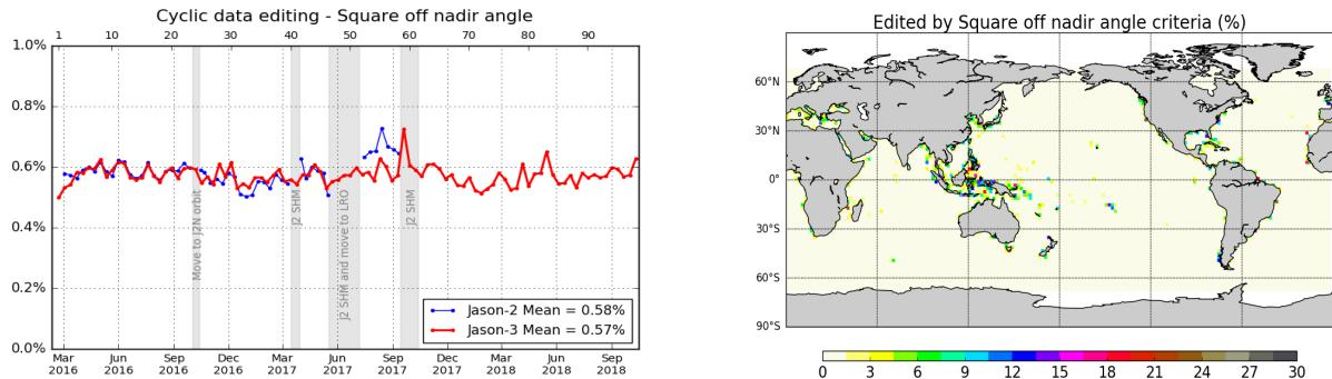
Figure 17 – Percentage of edited measurements by square off nadir angle threshold criterion. Left: Cycle per cycle monitoring compared with Jason-2. Right: Jason-3 averaged map from cycle 62 to 98.
