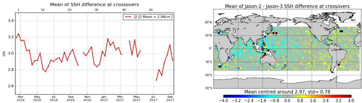
*Figure 5 – Cyclic monitoring of Jason-2 - Jason-3 SSH crossover differences mean (left) and map over cycle 1 to 58 (right). Only data with  $|latitude| < 50^\circ$ , bathymetry  $< -1000m$  and low oceanic variability were selected.*
