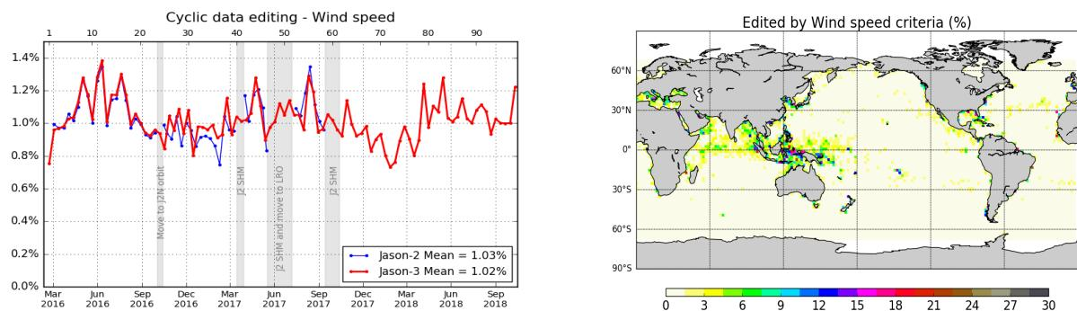
Figure 14 – Percentage of edited measurements by wind speed threshold criterion. Left: Cycle per cycle monitoring compared with Jason-2. Right: Jason-3 averaged map from cycle 62 to 98.
