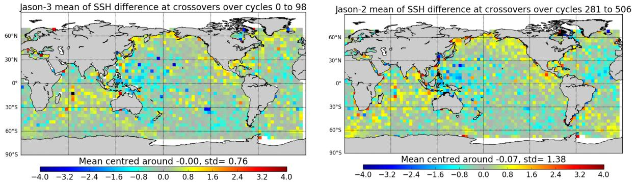
Figure 44 – Map of SSH crossovers differences mean for Jason-3 cycle 0 to 98(left) and for Jason-2 cycle 281 to 506 (right)
