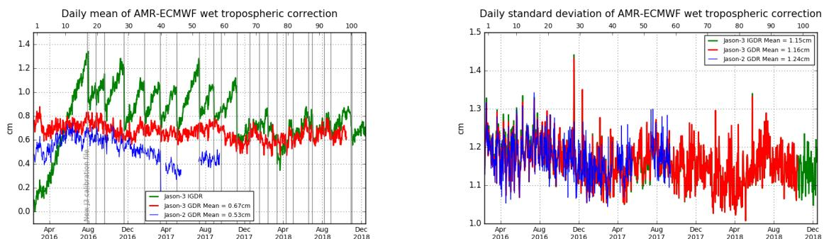
Figure 37 – Daily monitoring of AMR minus ECMWF model wet tropospheric correction. mean (left) and standard deviation (right)
