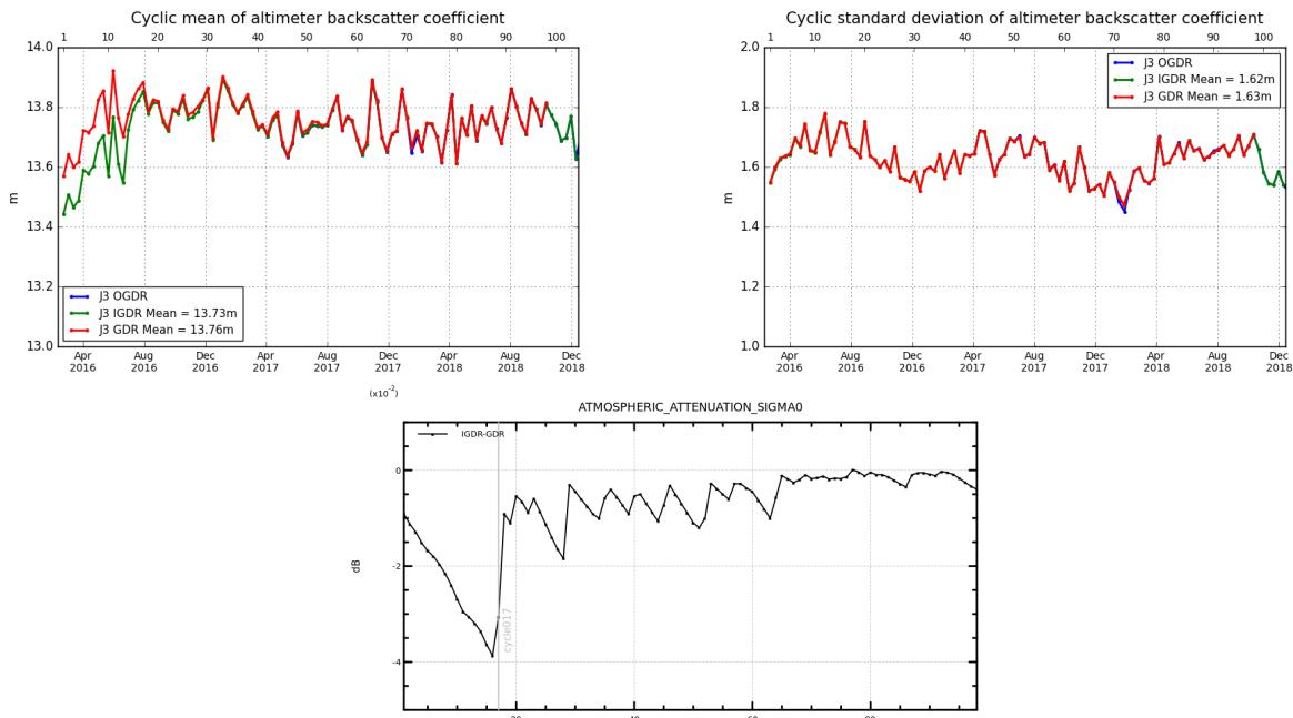
Figure 27 – Top: Cyclic monitoring of backscatter coefficient for Jason-3 (Ku-band) OGDR/IGDR/GDR. Bottom: difference of atmospheric attenuation applied to sigma0 between IGDR and GDR products.
