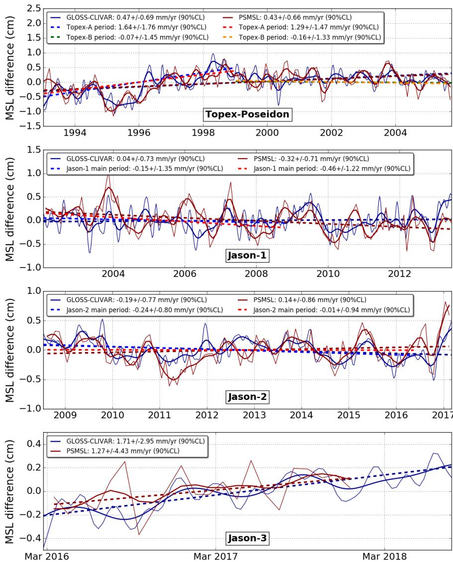
Figure 52 – Evolution of GMSL differences between altimeter and tide gauges for reference missions used in the GMSL indicator calculation (TOPEX/Poseidon, Jason-1, Jason-2 and Jason-3) with the GLOSS/CLIVAR network (blue line) and the PSMSL network (red line). Signal lower than 2 months and annual signals have been removed. The blue dashed line is the trend obtained applying a generalized least square method.
