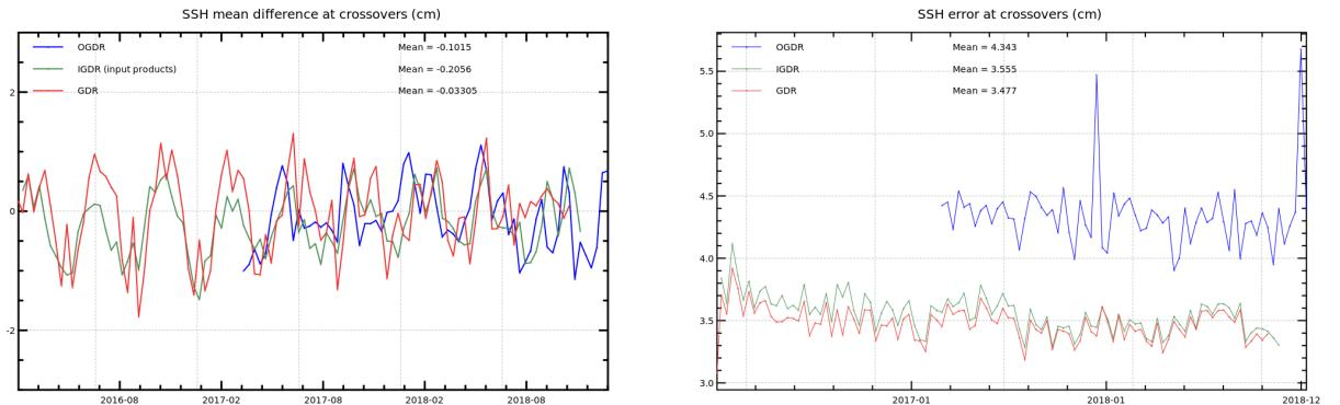
Figure 4 – Monitoring of SSH difference at crossovers for Jason-3 OGDR, IGDR and GDR. Mean of difference (**left**) and error at crossovers (**right**). Only data with  $|latitude| < 50^\circ$ , bathymetry  $< -1000m$  and low oceanic variability were selected.
