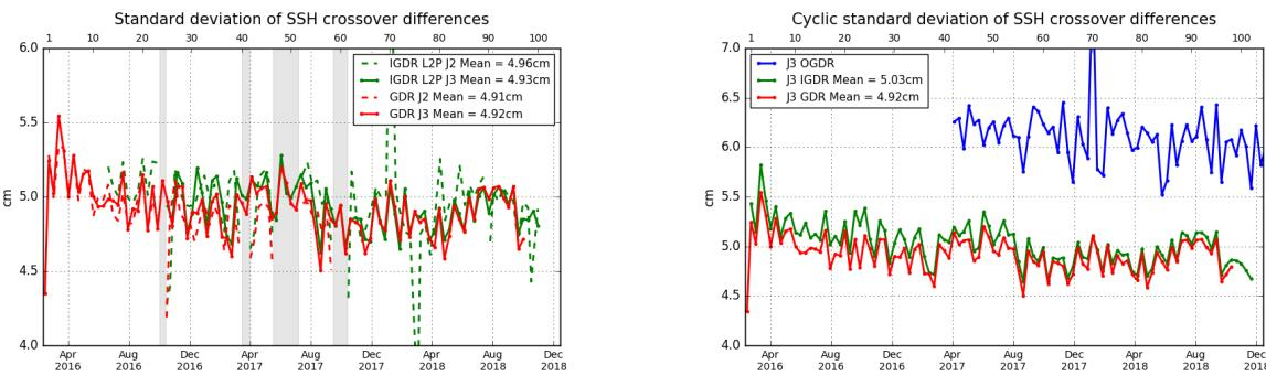
Figure 46 – Cycle by cycle standard deviation of SSH crossover differences for Jason-2 and Jason-3 (left), and for Jason-3 using OGDRs, IGDRs and GDRs (right). Only data with  $|latitude| < 50^\circ$ , bathymetry  $< -1000m$  and low oceanic variability were selected.
