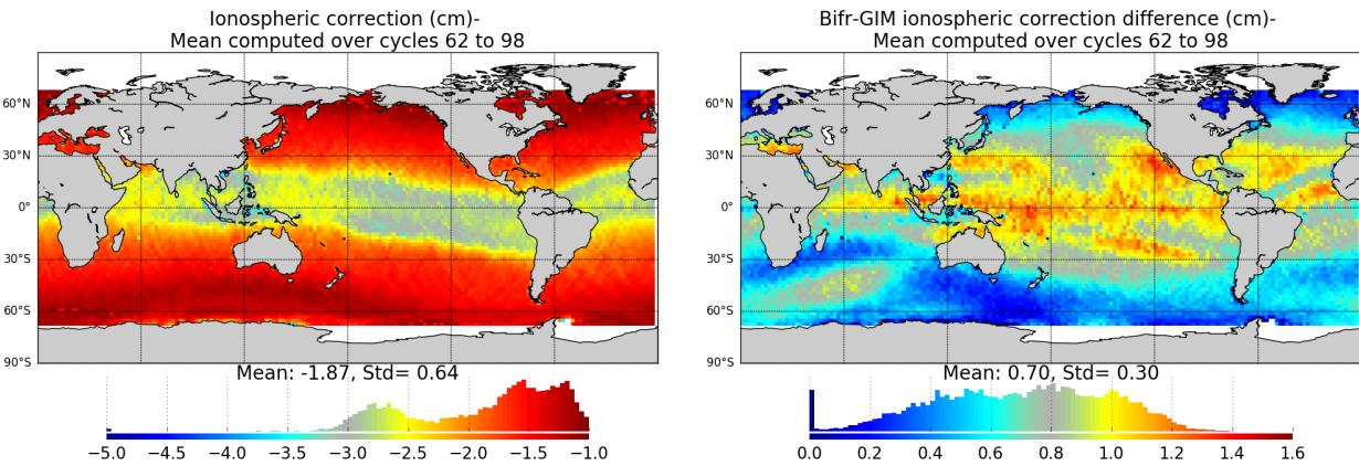
Figure 34 – Left: Map of ionospheric correction for Jason-3 averaged over cycles 62 to 98. Right: Map of dual-frequency minus GIM ionospheric correction solutions.
