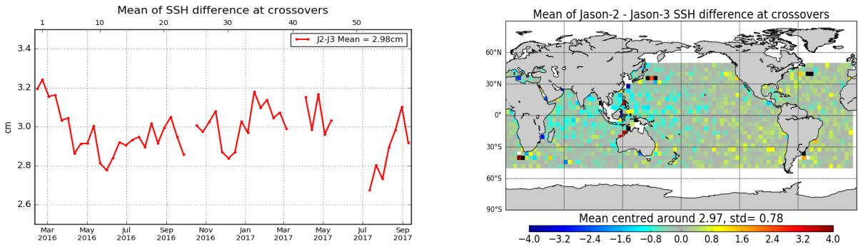
Figure 45 – Cyclic monitoring of Jason-2 - Jason-3 SSH crossover differences mean (left) and map over cycle 1 to 58 (right). Only data with  $|latitude| < 50^\circ$ , bathymetry  $< -1000m$  and low oceanic variability were selected.
