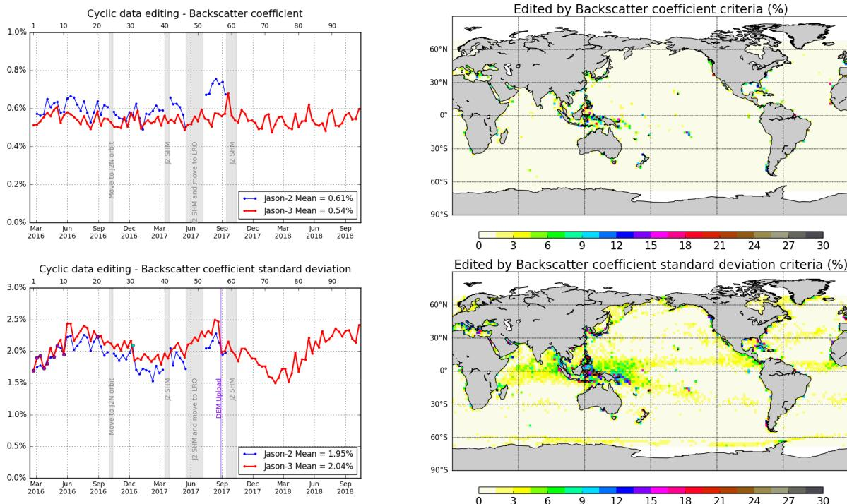
*Figure 11 – Percentage of edited measurements by backscatter coefficient threshold criterion (top) and by 20Hz backscatter coefficient standard deviation threshold criteria (bottom). Cycle per cycle monitoring compared with Jason-2 (left, Jason-2 DEM cycle in cyan. Jason-3 median tracker cycles in purple) and Jason-3 averaged map from cycle 62 to 98 (right).*
