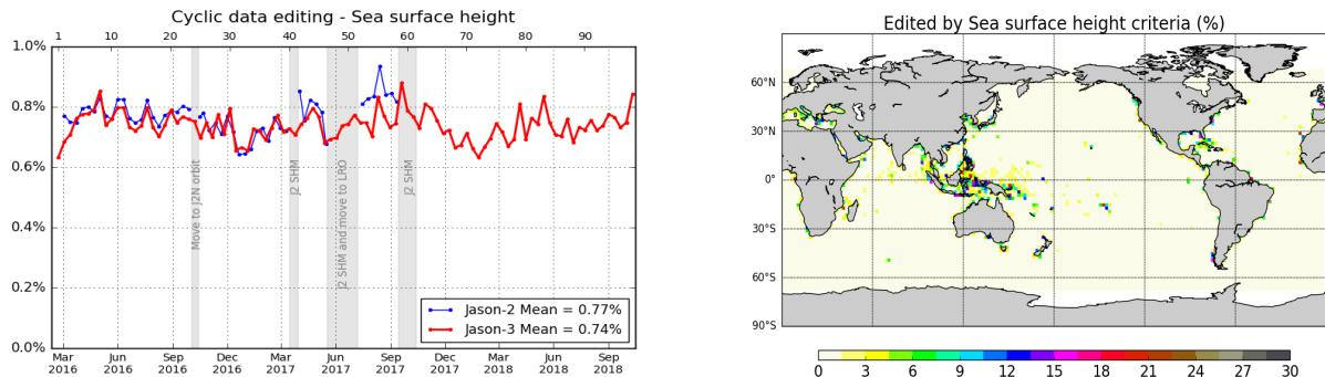
Figure 18 – Percentage of edited measurements by sea surface height threshold criterion. Left: Cycle per cycle monitoring compared with Jason-2. Right: Jason-3 averaged map from cycle 62 to 98.
