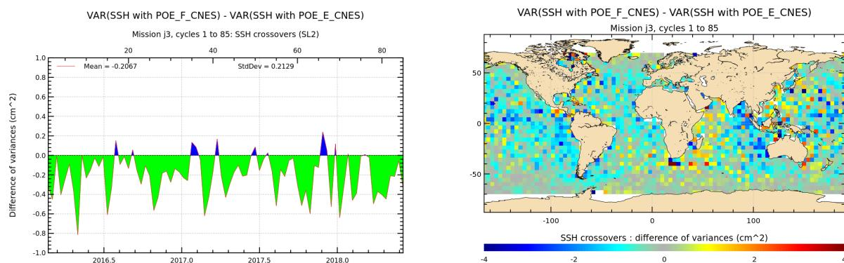
Figure 61 – difference of variance at crossovers between CNES POE-E and CNES POE-F (OceanTide=FES14B, Ionospheric correction=filtered dual-freq. alti)
