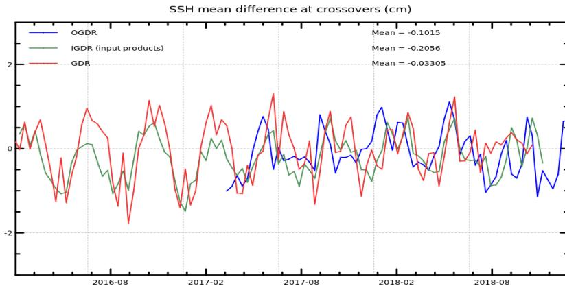
Figure 42 – Monitoring of mean of Jason-3 SSH crossover differences for OGDRs, IGDRs and GDRs. Only data with  $|latitude| < 50^\circ$ , bathymetry  $< -1000m$  and low oceanic variability were selected.
