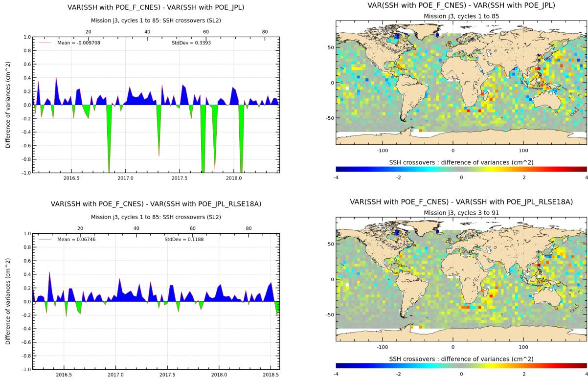
*Figure 62 – difference of variance at crossovers between CNES POE-F or JPL solutions (OceanTide=FES14B, Ionospheric correction=filtered dual-freq. alti). **top:** with operational JPL POE, **bottom:** with release18a JPL POE*
