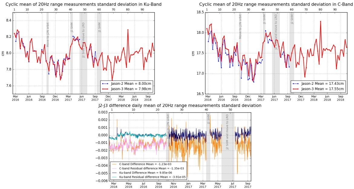
**Figure 22 – Top:** Cyclic monitoring of elementary 20 Hz range measurements standard deviation for Jason-2 and Jason-3 for Ku-band and C-band. **Bottom:** Jason-2 - Jason-3 difference daily monitoring of elementary 20 Hz range measurements standard deviation.
