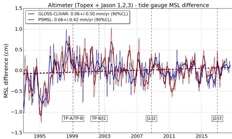
Figure 53 – Evolution of global MSL differences from altimeter / tide gauges comparisons (GLOSS/CLIVAR and PSMSL network) from TOPEX/Poseidon, Jason-1, Jason-2 and Jason-3 L2P products linked together.
