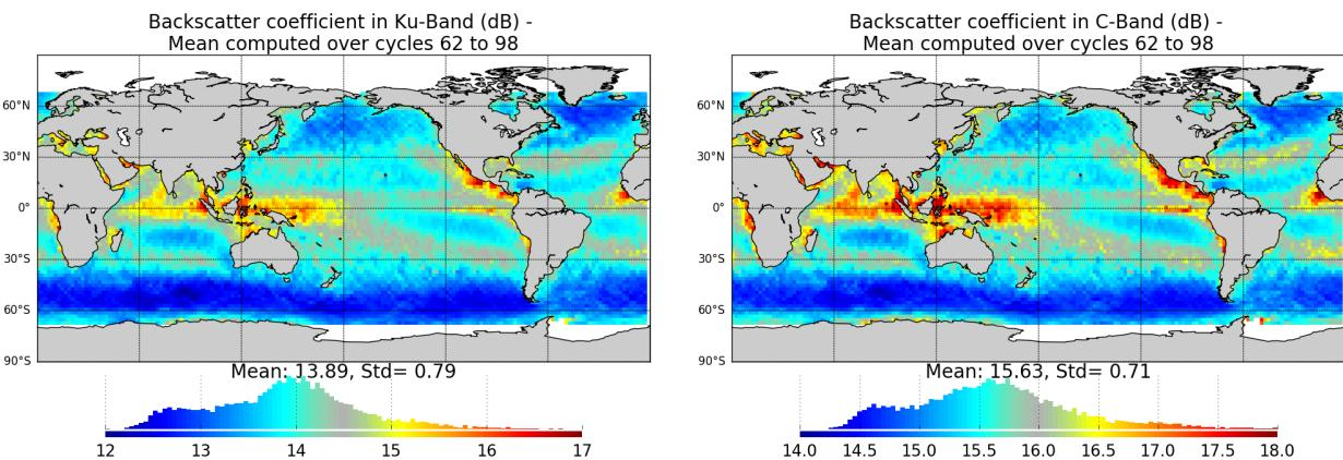
**Figure 29 –** Map of backscatter coefficient for Jason-3 averaged over cycles 62 to 98, in Ku-band (left) and in C-band (right).
