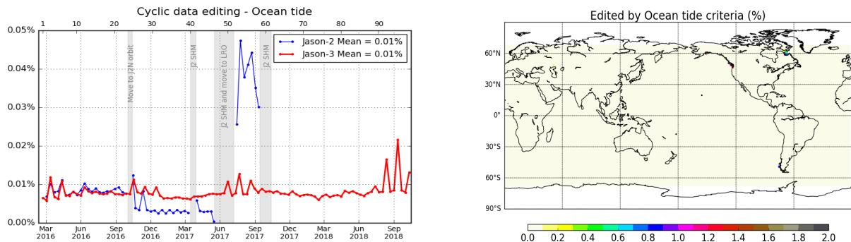
*Figure 16 – Percentage of edited measurements by ocean tide threshold criterion. Left: Cycle per cycle monitoring compared with Jason-2. Right: Jason-3 averaged map from cycle 62 to 98.*
