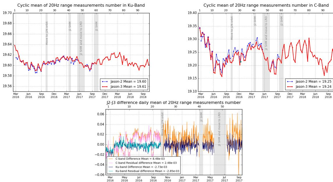
Figure 20 – **Top:** Cyclic monitoring of number of elementary 20 Hz range measurements for Jason-2 and Jason-3 for Ku-band and C-band. **Bottom:** Jason-2 - Jason-3 difference daily monitoring of elementary 20 Hz range measurements number (until september 2017).
