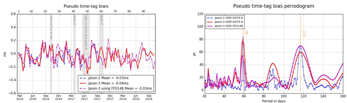
Figure 47 – Monitoring (left) and periodogram (right) of pseudo time-tag bias estimated cycle by cycle from GDR products for Jason-2 and Jason-3
