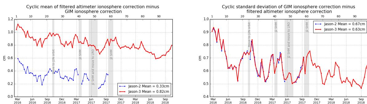
Figure 35 – Cyclic monitoring of GIM ionosphere correction minus filtered altimeter ionosphere correction for Jason-2 and Jason-3. Left: mean, right: standard deviation.
