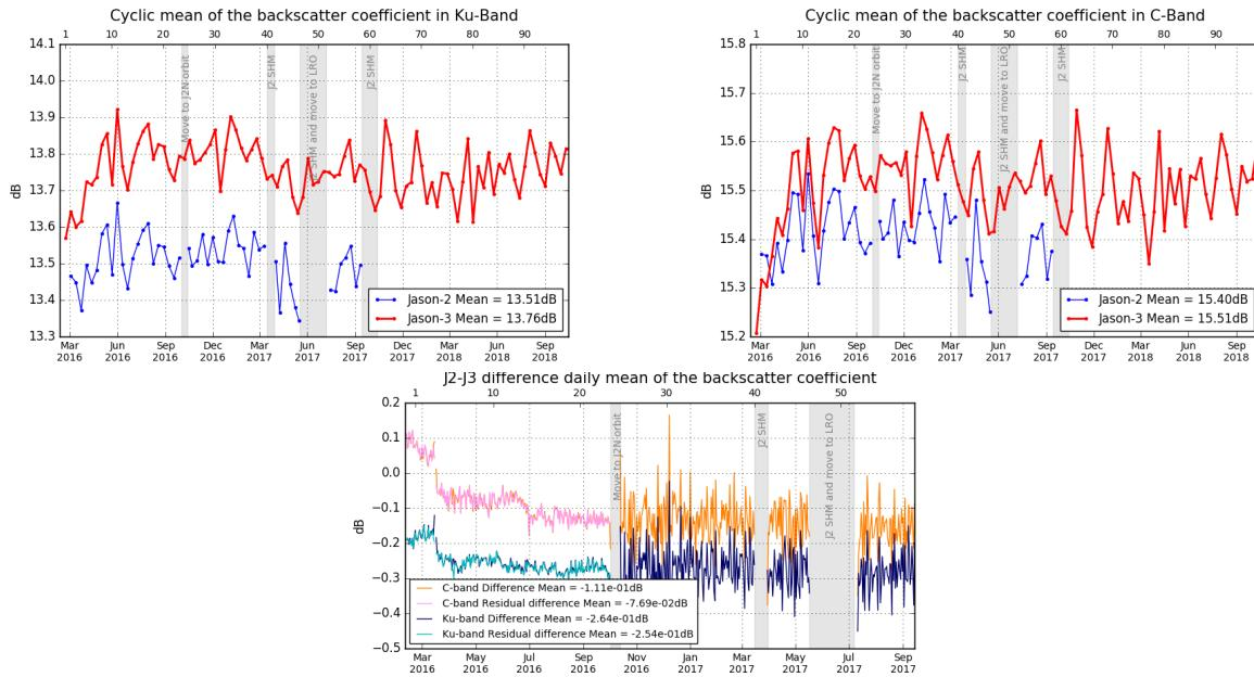
**Figure 28 – Top:** Cyclic monitoring of backscatter coefficient for Jason-2 and Jason-3 for Ku-band (left) C-band (right). **Bottom:** daily monitoring of Jason-2 - Jason-3 GDR difference of the backscatter coefficient.
