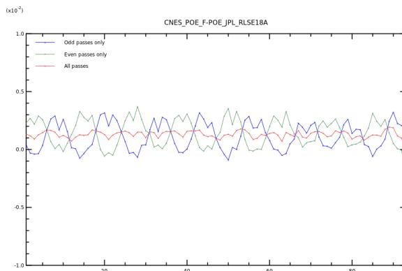
**Figure 64 – Difference between CNES POE-F and JPL POE release18a, separating odd and even passes**
