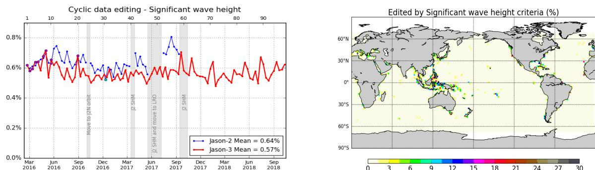
Figure 10 – Percentage of edited measurements by SWH threshold criterion. Left: Cycle per cycle monitoring compared with Jason-2 (Jason-2 DEM cycle in cyan. Jason-3 median tracker cycles in purple.) Right: Jason-3 averaged map from cycle 62 to 98 .
