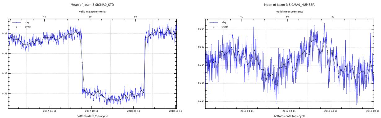
*Figure 56 – Left: Mean per day (blue) or per cycle (black) of standard deviation of sigma0 (left) and number of 20Hz measurements used to compute 1Hz sigma0 (right).*
