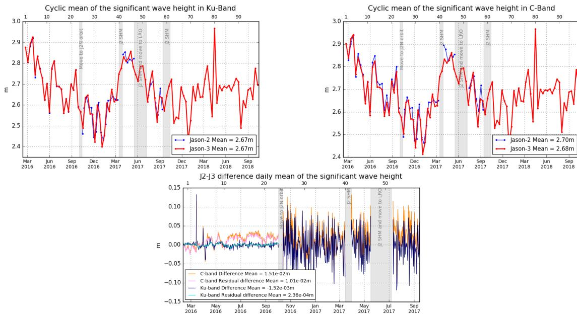
Figure 31 – Cyclic monitoring of significant wave height for Jason-2 and Jason-3 for Ku-band (left) and for C-band (right). Jason-2 - Jason-3 difference daily monitoring of significant wave height (bottom).
