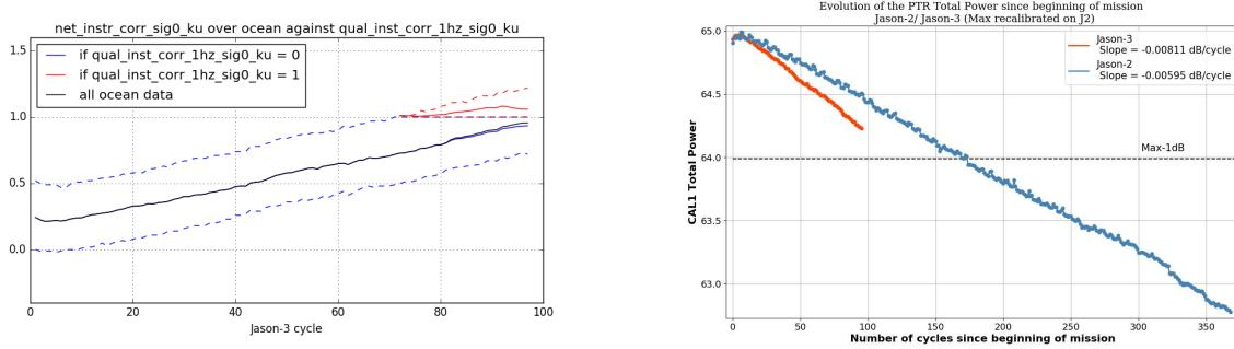
Figure 54 – Left: Jason-3 net\_instr\_corr\_sig0\_ku flag. Right: Jason-2 and Jason-3 evolution of PTR power.
