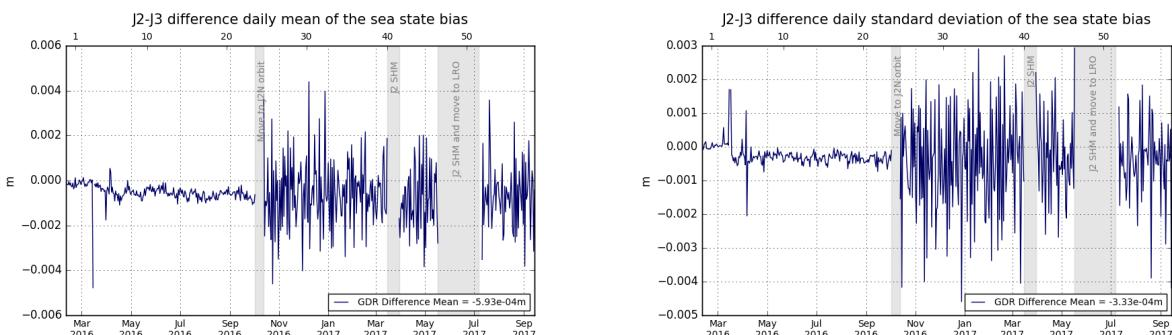
Figure 41 – Jason-2 - Jason-3 difference daily monitoring of the sea state bias mean (left) and standard deviation (right).
