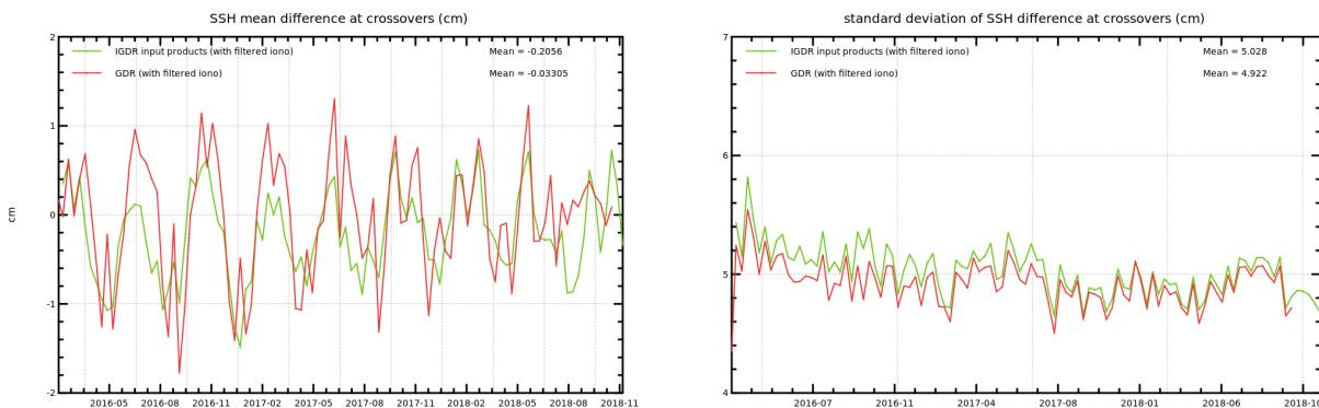
Figure 57 – Mean and standard deviation of SSH difference at crossovers with geographical selection for Jason-3 GDR and IGDR reference data (using ocean tide sol1 = GOT4.8)
