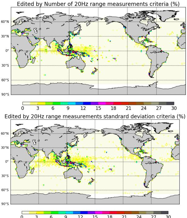
Figure 9 – Percentage of edited measurements by 20Hz range measurements threshold criterion (top) and by 20Hz range measurements standard deviation threshold criteria (bottom). Cycle per cycle monitoring compared with Jason-2 (left) and Jason-3 averaged map from cycle 62 to 98 (right).
