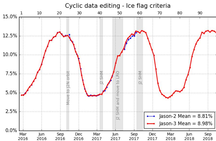
Figure 6 – Cycle per cycle monitoring of the percentage of edited measurements by ice flag criterion.
