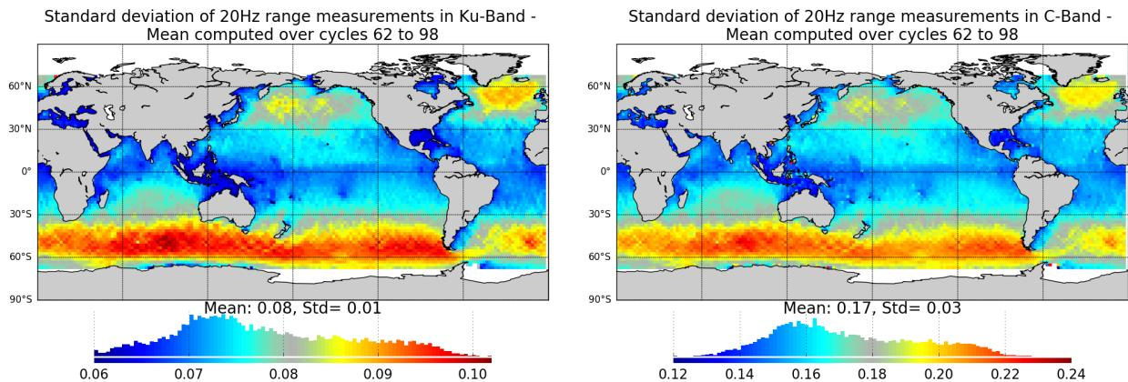
**Figure 23 –** Map of 20 Hz range measurements standard deviation for Jason-3 averaged over cycles 62 to 98, in Ku-band (left) and in C-band (right).
