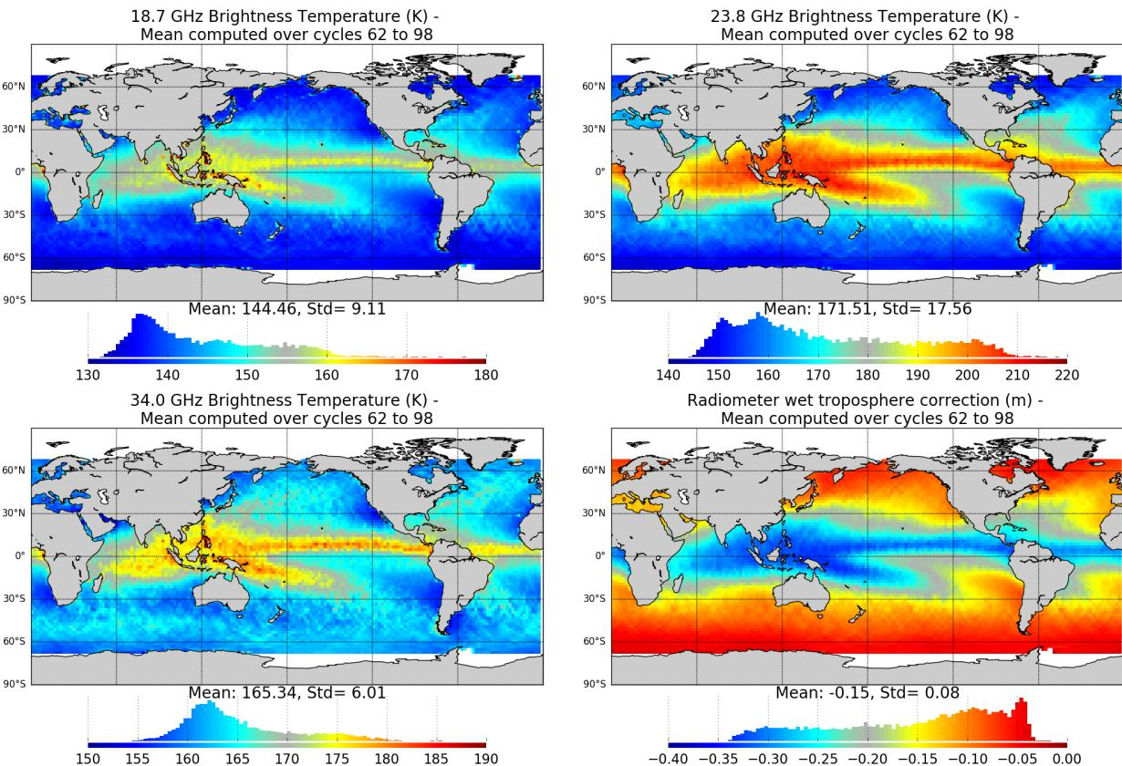
Figure 36 – Map of Jason-3 brightness temperatures averaged over cycles 62 to 98: 18.7 Ghz channel (top left), 23.8 Ghz channel (top right) and 34.0 Ghz channel (bottom left). Map of AMR wet troposphere correction for Jason-3 averaged over cycles 62 to 98 (bottom right)
