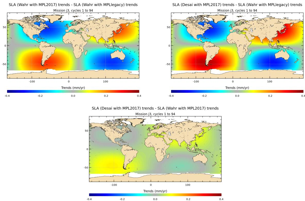
*Figure 67 – Difference of trends for : Top left: SLA using Wahr85 with MPL2017 - SLA using GDR (Wahr85 and MPL legacy), Top right: SLA using Desai2015 with MPL2017 - SLA using GDR (Wahr85 and MPL legacy), Bottom: SLA using Wahr85 with MPL2017 - SLA using Desai2015 with MPL2017*
