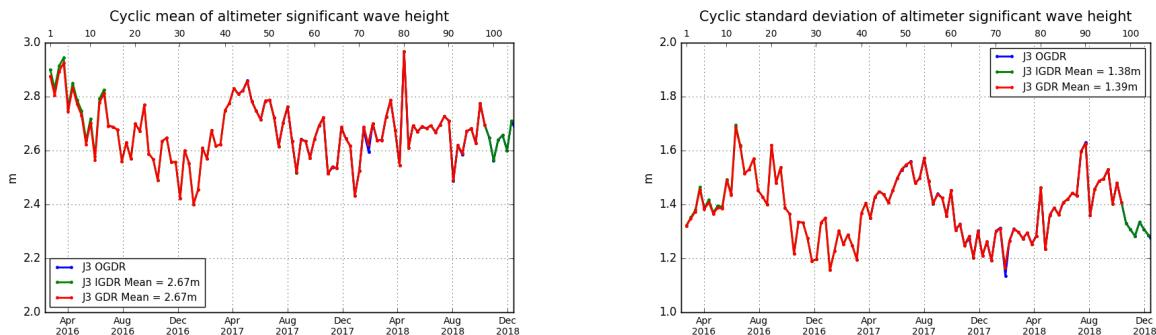
Figure 30 – Cyclic monitoring of significant wave height for Jason-3 (Ku-band) OGDR/IGDR/GDR.
