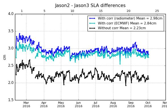
Figure 48 – Daily monitoring of SSH bias between Jason-2 and Jason-3 before Jason-2 moved to interleaved ground-track in October 2016: SSH bias without applying geophysical corrections (**black**) and with corrections using radiometer wet troposphere correction (**blue**) or using ECMWF model wet troposphere correction (**cyan**).
