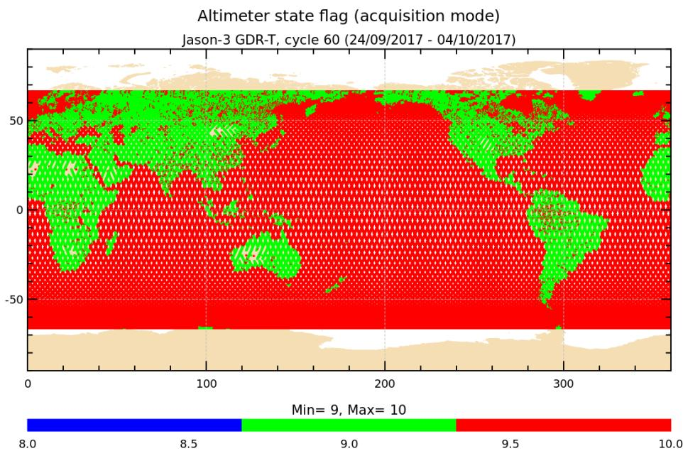
*Figure 1 – Acquisition mode for cycle 060 (identical to acquisition mode automatic switch for cycles 6, 9, 11-19, 21-56,58-98). 8 = autonomous acquisition / tracking, 9 = autonomous DIODE acquisition / tracking, 10 = DIODE + Digital Elevation Model tracking*
