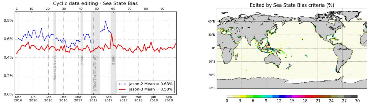
*Figure 15 – Percentage of edited measurements by sea state bias threshold criterion. Left: Cycle per cycle monitoring compared with Jason-2. Right: Jason-3 averaged map from cycle 62 to 98.*
