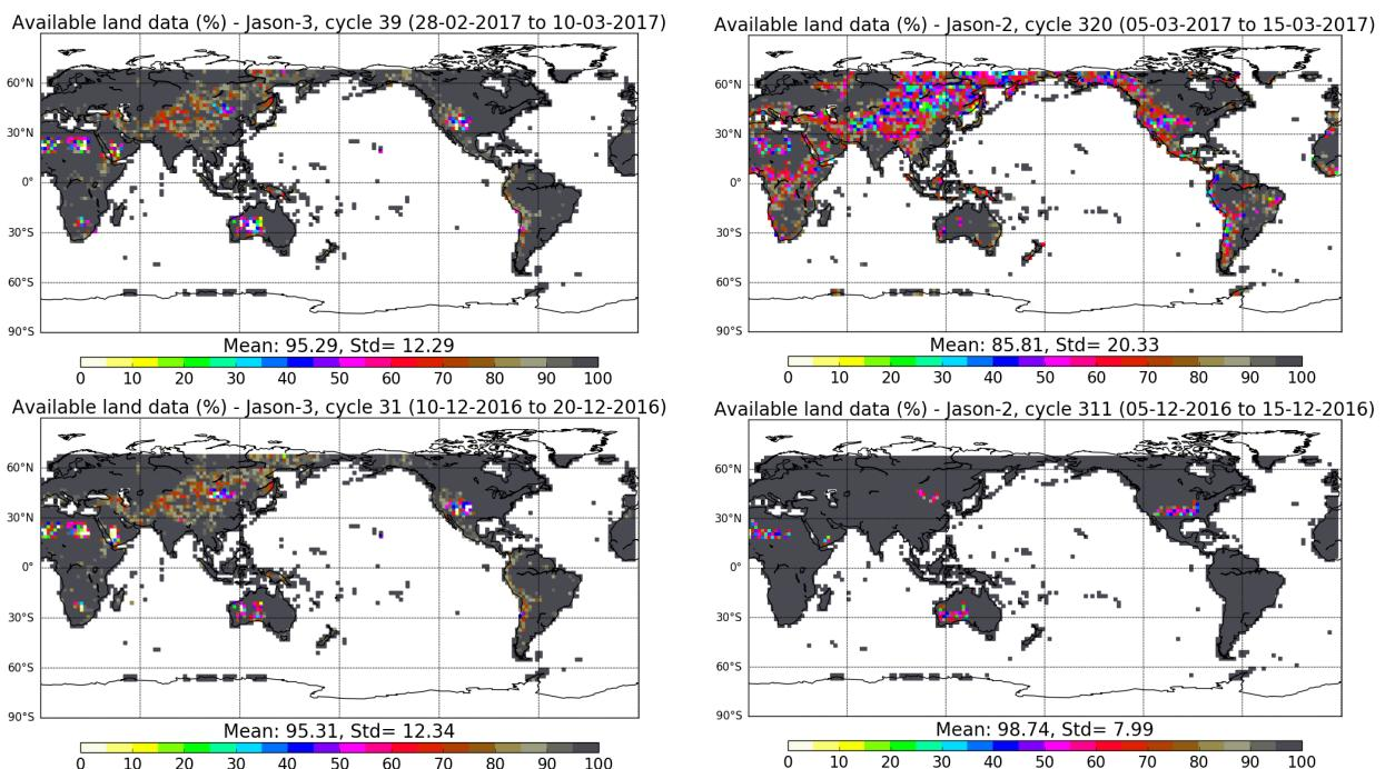
Figure 3 – Map of percentage of available measurements over land for Jason-3 (left) and for Jason-2 (right). **Top:** Jason-3 cycle 039 in DEM mode and Jason-2 cycle 320 in median mode. **Bottom:** Jason-3 cycle 031 in DEM mode and Jason-2 cycle 311 in DEM mode
