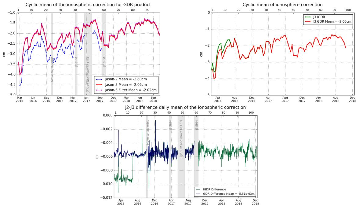
Figure 33 – Cyclic monitoring of ionospheric correction for Jason-2 and Jason-3. (left). Cyclic monitoring of Jason-3 ionospheric correction for IGDR and GDR data (right). Jason-2 - Jason-3 difference daily monitoring of ionospheric correction (bottom).
