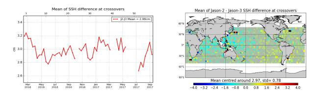
Figure 5 – Cyclic monitoring of Jason-2 - Jason-3 SSH crossover differences mean (left) and map over cycle 1 to 58 (right). Only data with  $|latitude| < 50^{\circ}$ , bathymetry < -1000m and low oceanic variability were selected.
