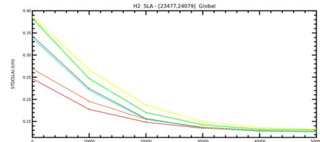
Fig 4: STD of the SLA along HY-2A tracks as a function of the distance to the coast, and using different MSS solution. (Latitudes  $> 60^\circ$  are excluded)
