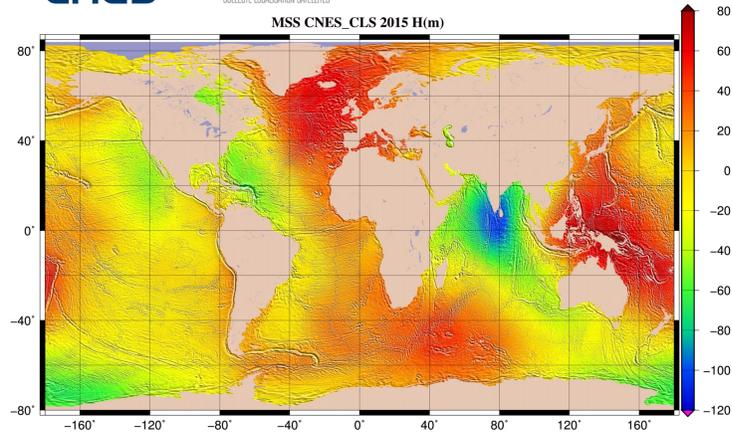
Fig 1: Mean Sea Surface CNES\_CLS 2015. Heights are in meter above T/P ellipsoid.
