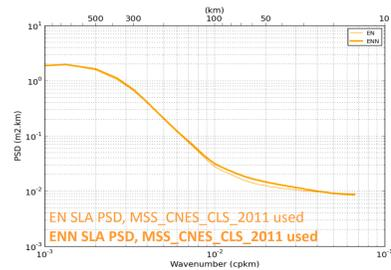
Fig 2: SLA PSD and SLAPSD ratio. Comparison of SLA along Envisat repetitive tracks (EN) and geodetic tracks (ENN). SLA PSD ratio along Jason-2 tracks is used as reference ratio.
