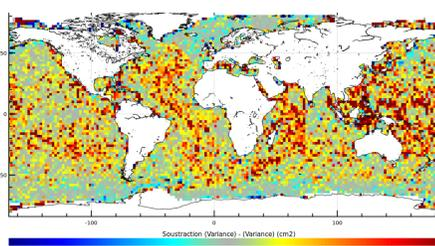
Fig 3a: Difference of the variance of the SLA selected on wavelength  $< 250$ km along HY-2A tracks when MSS\_CNES\_CLS\_2011 and MSS\_CNES\_CLS\_2015 is used. Statistics computed over year 2015.
