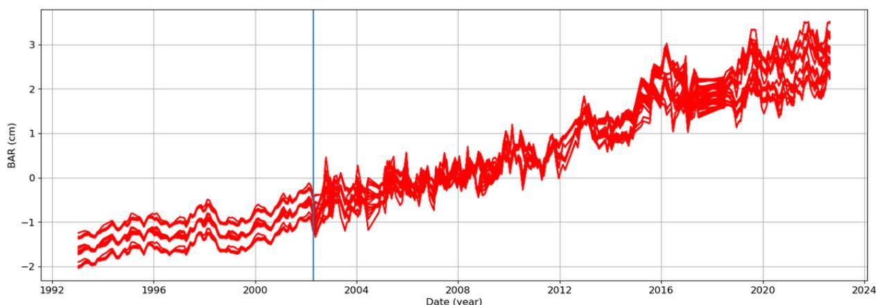
Figure 3 : Timeseries of all the solutions of the barystatic sea level after the concatenation. The removal of the annual signal was done prior to plotting. The vertical blue line represents the date at which the concatenation between GRACE and SLBC\_cci data is done.
