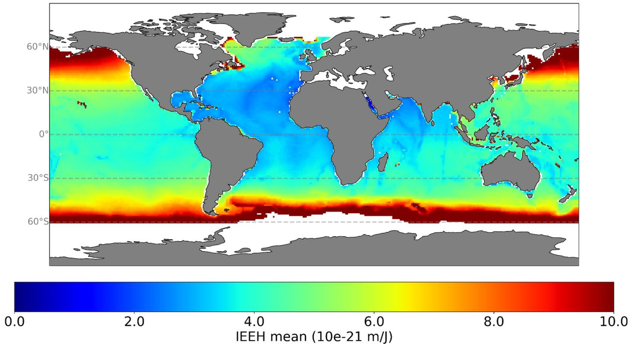
Figure 5 Time-mean of the Integrated Expansion Efficiency of Heat (IEEH) coefficients ( $10^{-21}$  m/J) (1x1 degree).
