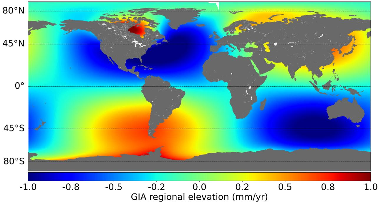
Figure 4 Regional grid of the GIA correction applied to altimetry sea level grids in MOHeaCAN processing chain (Spada and Melini, 2019)
