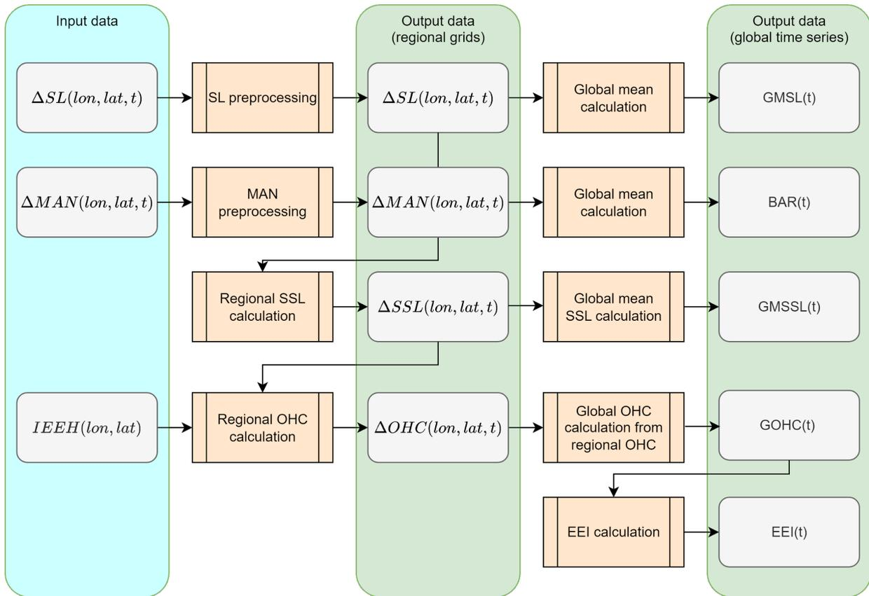
Figure 6 Overview of the MOHeaCAN processing chain. Variables are given with their dimensions (lon: longitude, lat: latitude, t: time). Global mean time series ( $GMSL$ ,  $BAR$ ,  $GMSL$ ) are computed but do not intervene in the  $GOHC/EEI$  calculation afterwards.
