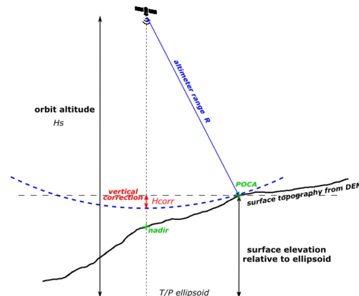
**Figure 2: Schematic illustration of the measurement relocation processing**
