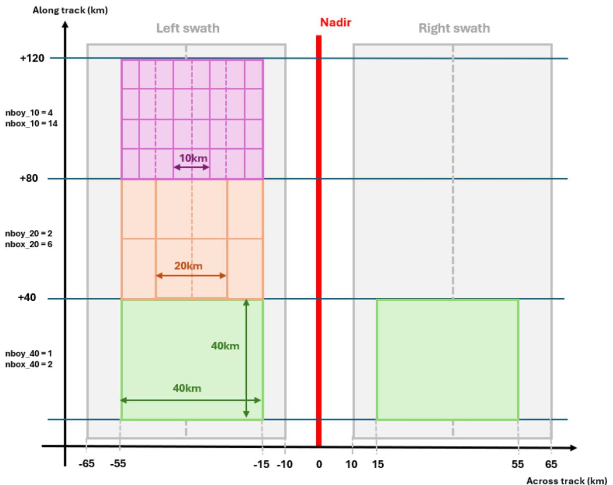
Figure 1 Schematic representation of the different spectral resolutions within the SWOT swath
