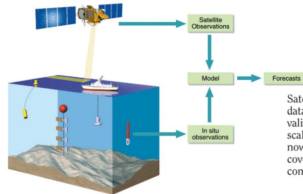
Satellite measurements are complemented by *in situ* data that enable us to plumb the ocean depths and validate and calibrate satellite instruments. Large-scale international programmes such as ARGO are now taking shape to provide the widest possible coverage of the oceans by *in situ* instruments, to complement spaceborne programmes.
