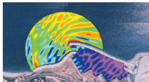
Forecasting swell helps to design breakwaters to reduce wave heights in harbours.
