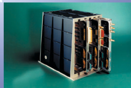
POSEIDON-2 altimeter processing unit (Alcatel) - Flight model.
