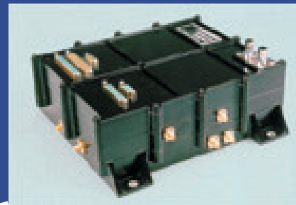
DORIS receiver (Thomson-Detexis) - Flight model.
