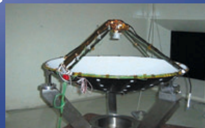
Altimeter antenna (Alcatel) - Flight model in preparation for thermal and mechanical tests.
