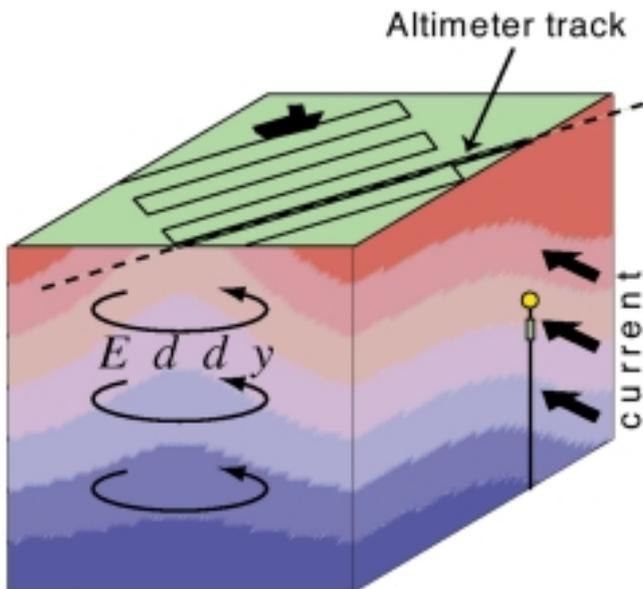
Figure 2: Using repeated altimeter tracks for monitoring eddies and inter-basin flows, in combination with ship surveys and current meters. [Here shifts in constant density layers (colored) illustrate the position of an eddy and a strong current].
