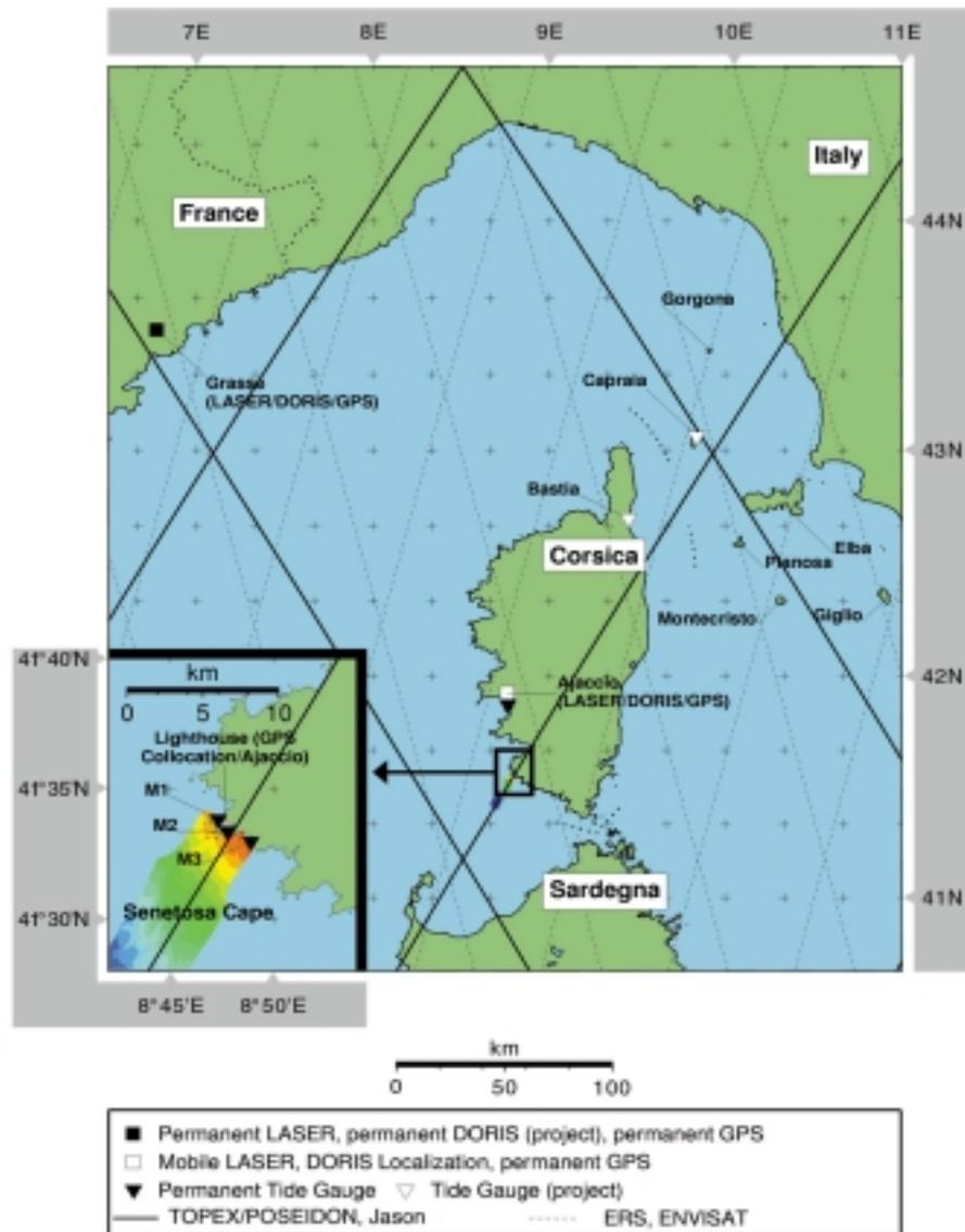
**Figure 1: Senetosa/Capraia calibration site. The surface in color, near Cap Senetosa (southern Corsica), represents the geoid determined with a Catamaran GPS.**
